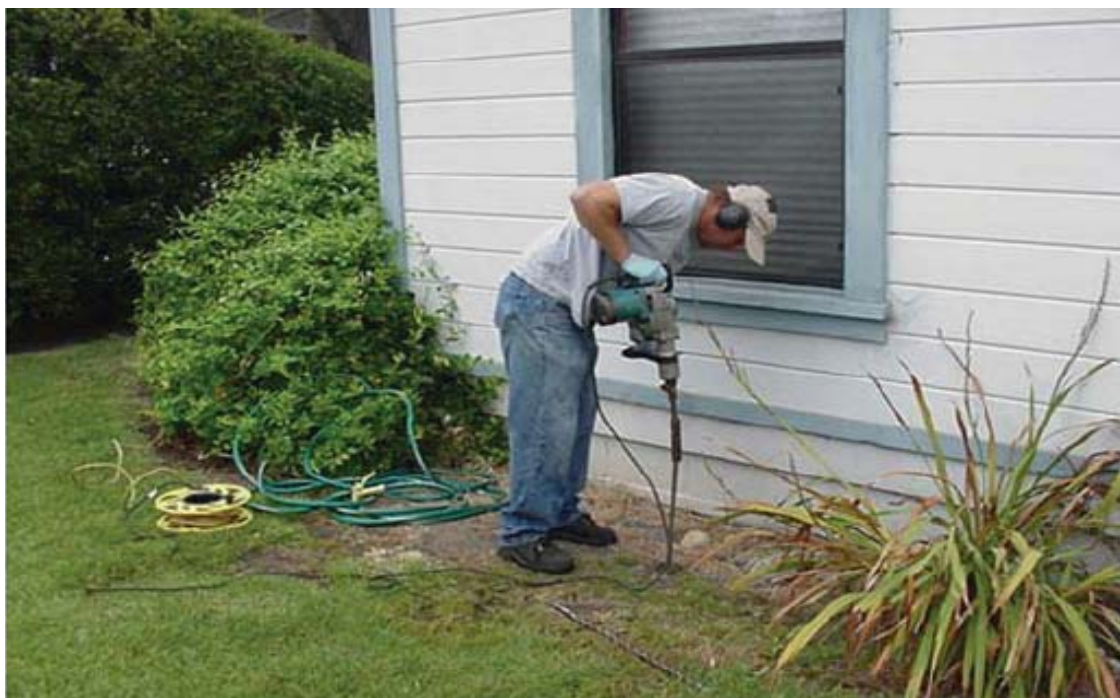
Figure 2. Installation of Soil Gas Probe Near a House. Soil gas probes are a primary method of collecting samples to measure soil-gas chemical concentrations.
