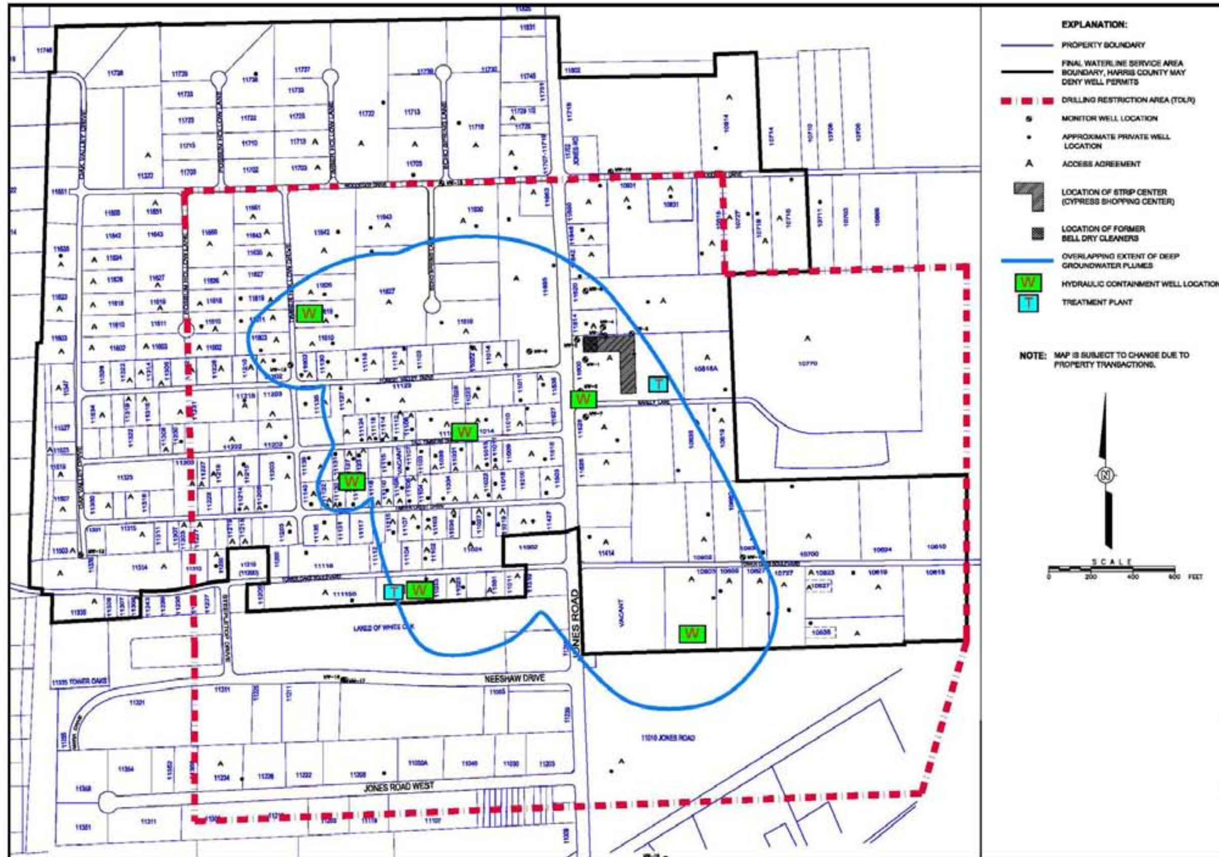
Figure 10 – Hydraulic Containment / Pump and Treat
