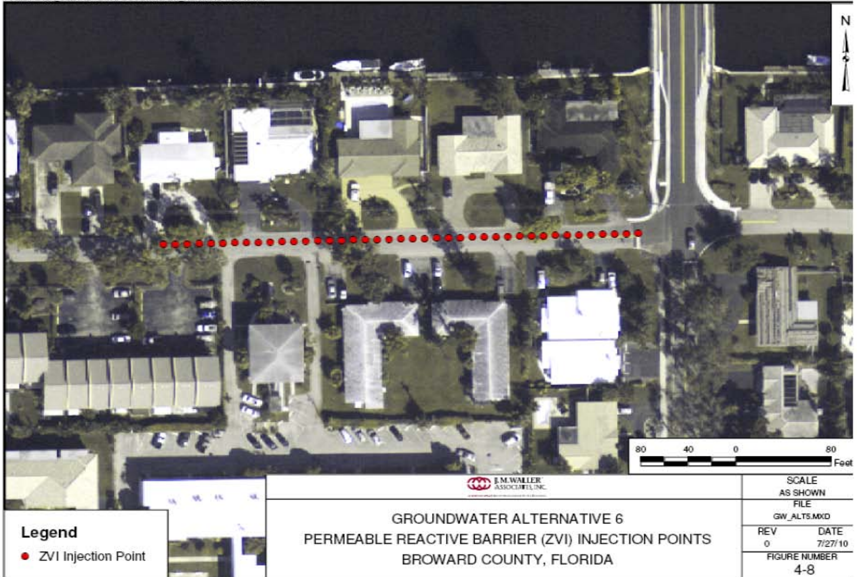
Figure 22 – Alternative GW- 6 Permeable Reactive Barrier
