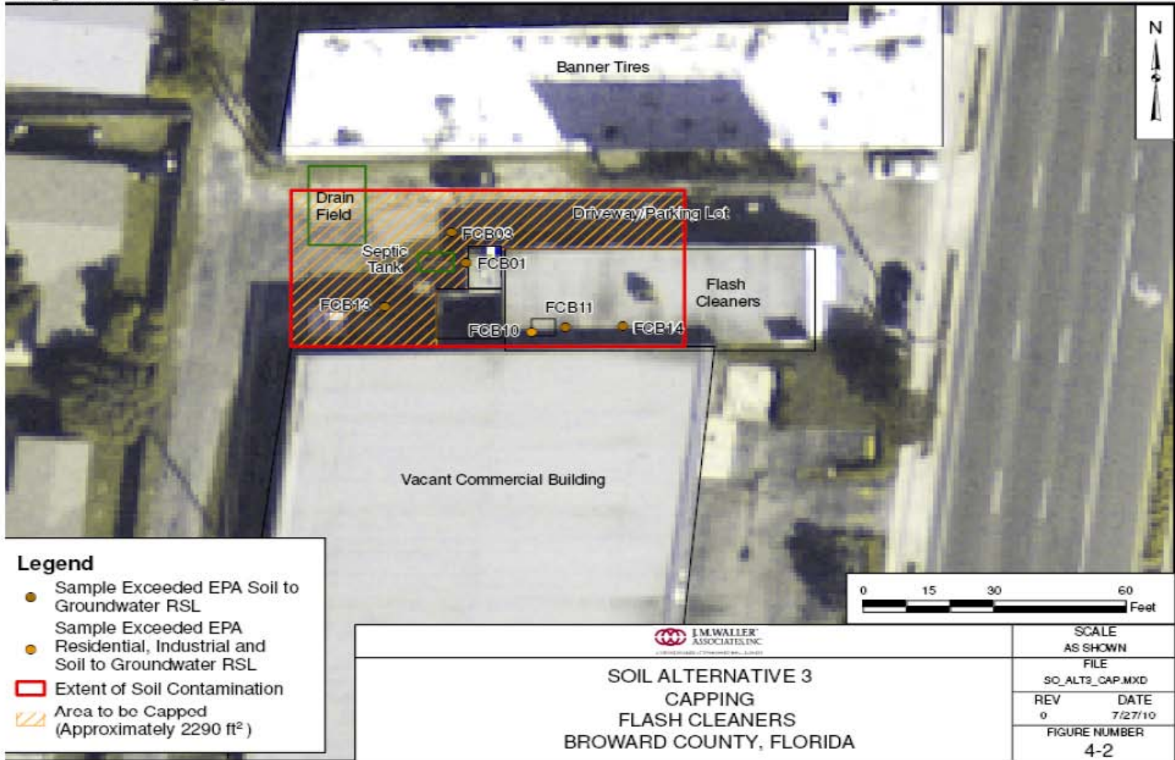
Figure 2 – Alternative S-3 Area of Capping
