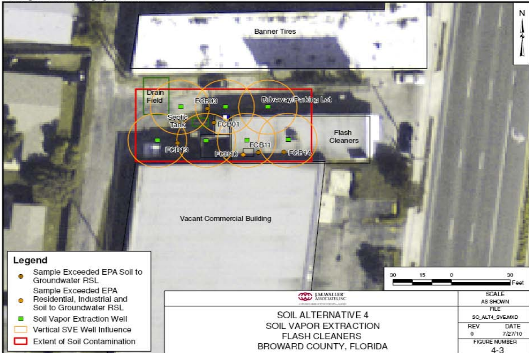
Figure 3 – Alternative S-4 Soil Vapor Extraction
