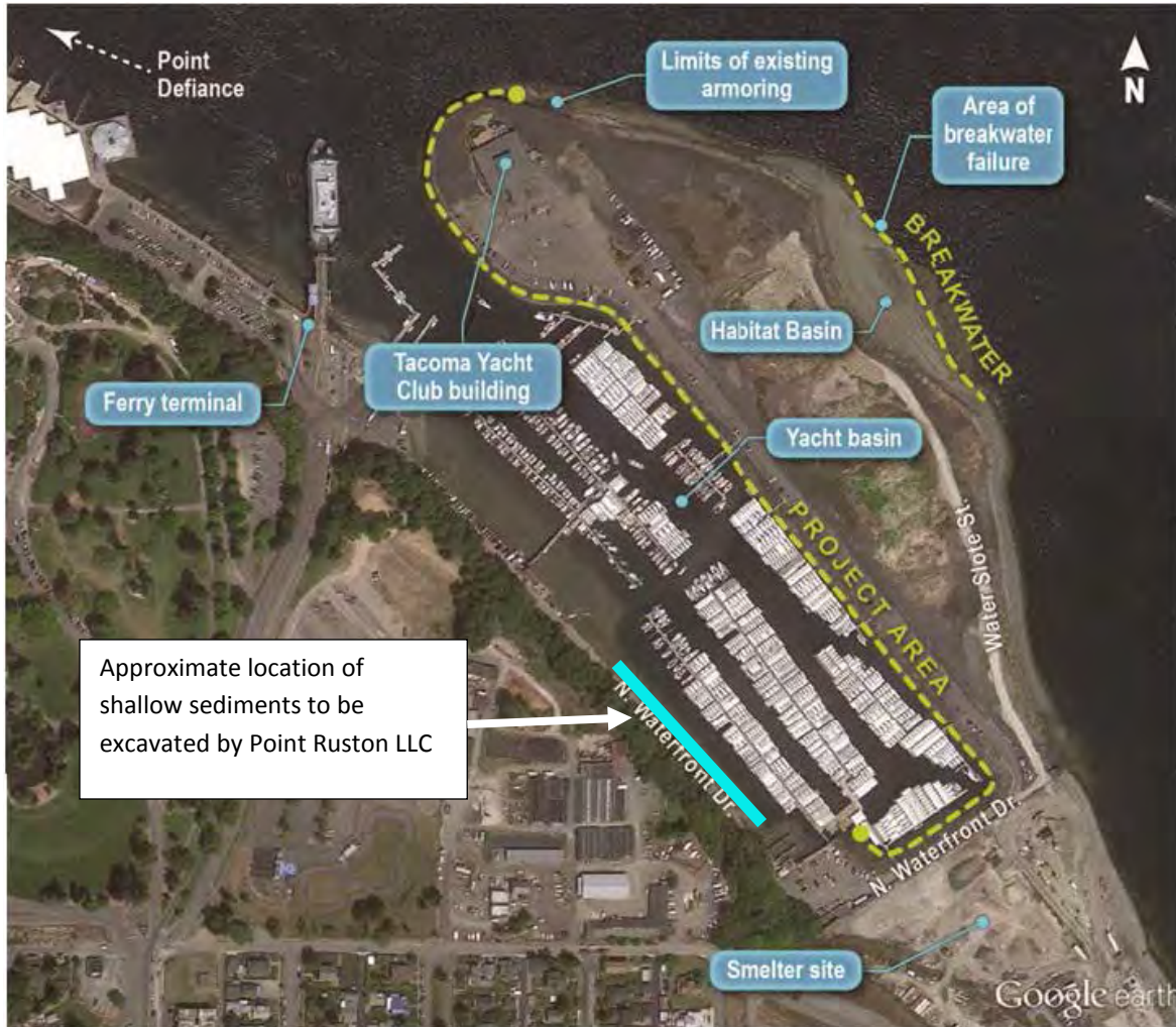
Figure 5-7. Approximate Location of Shallow Yacht Basin Sediments for Excavation
