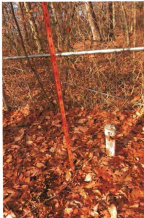
Monitoring well at Landfill No. 2.
