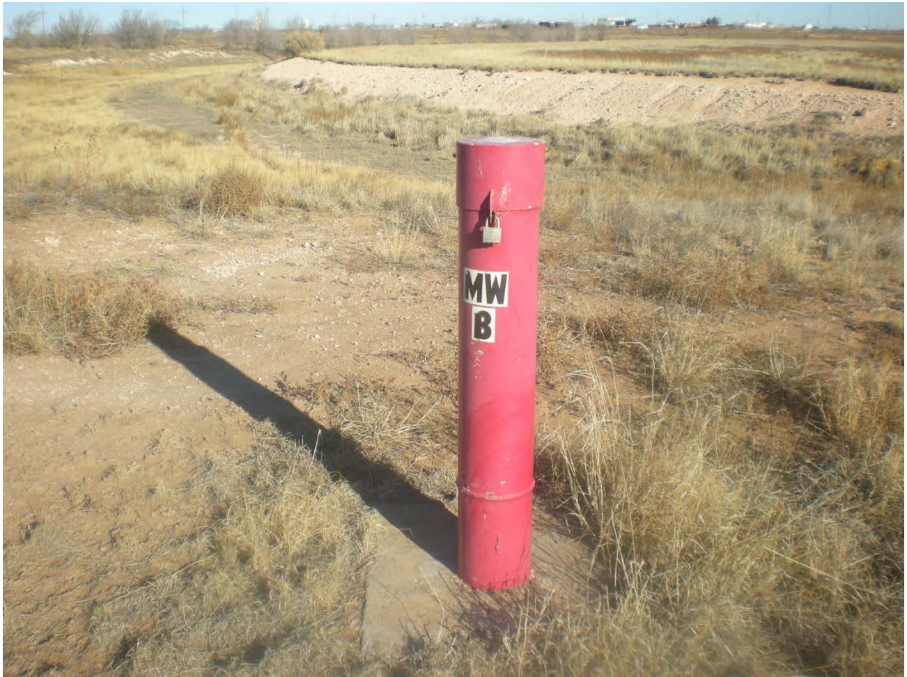
Photograph Number: 7 Photographer: Sabino Rivera Location: ATSF-Clovis Superfund Site Subject: View of Monitor Well B City: Clovis State: New Mexico Date: January 17, 2013
