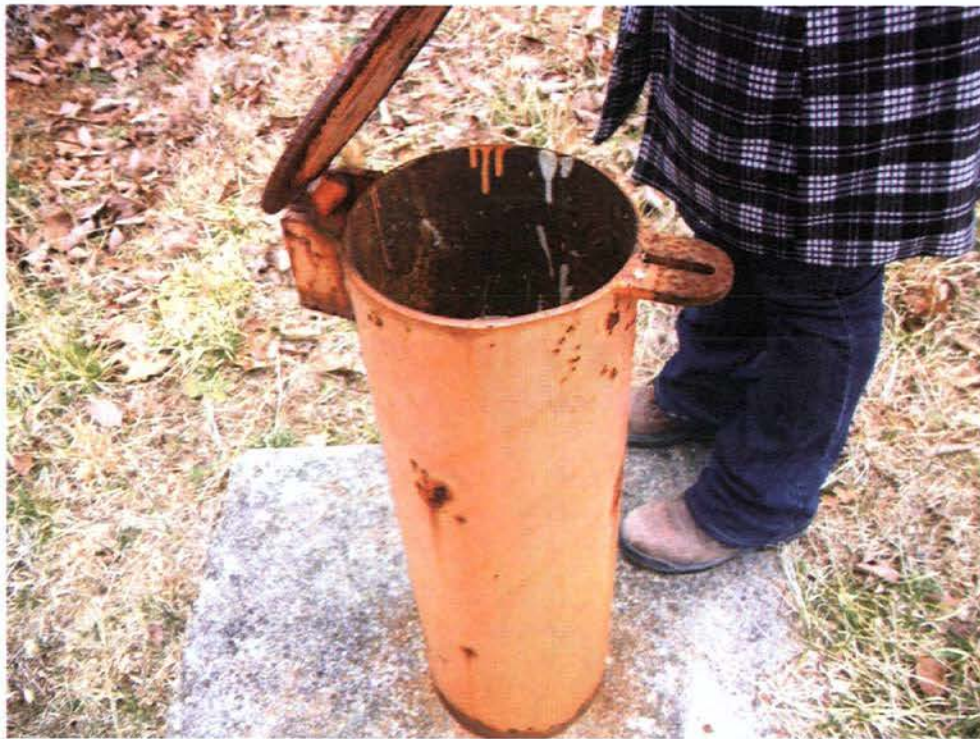
Photo: 231 Date: 02/28/13 Description: At monitoring well, MW-3B. Well protective casing missing lock. Photographer: Rich Opem
