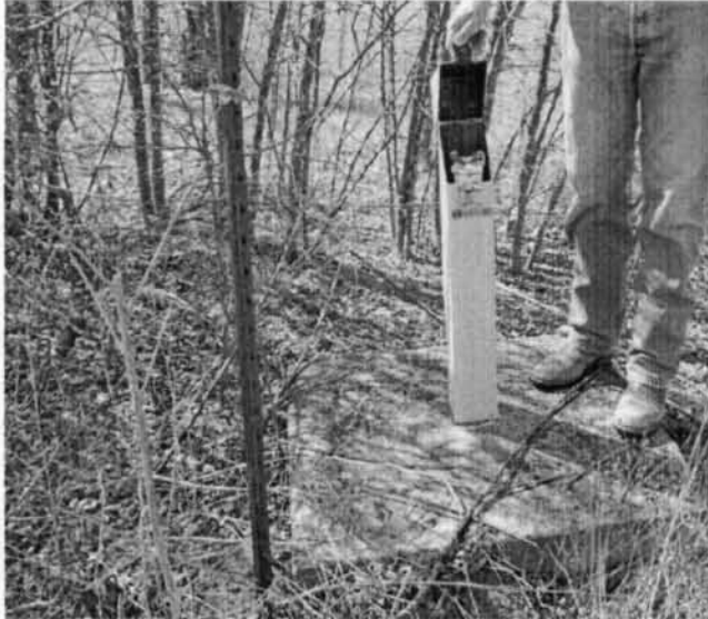
Photo 21. MW-33-90, well is missing the lock
