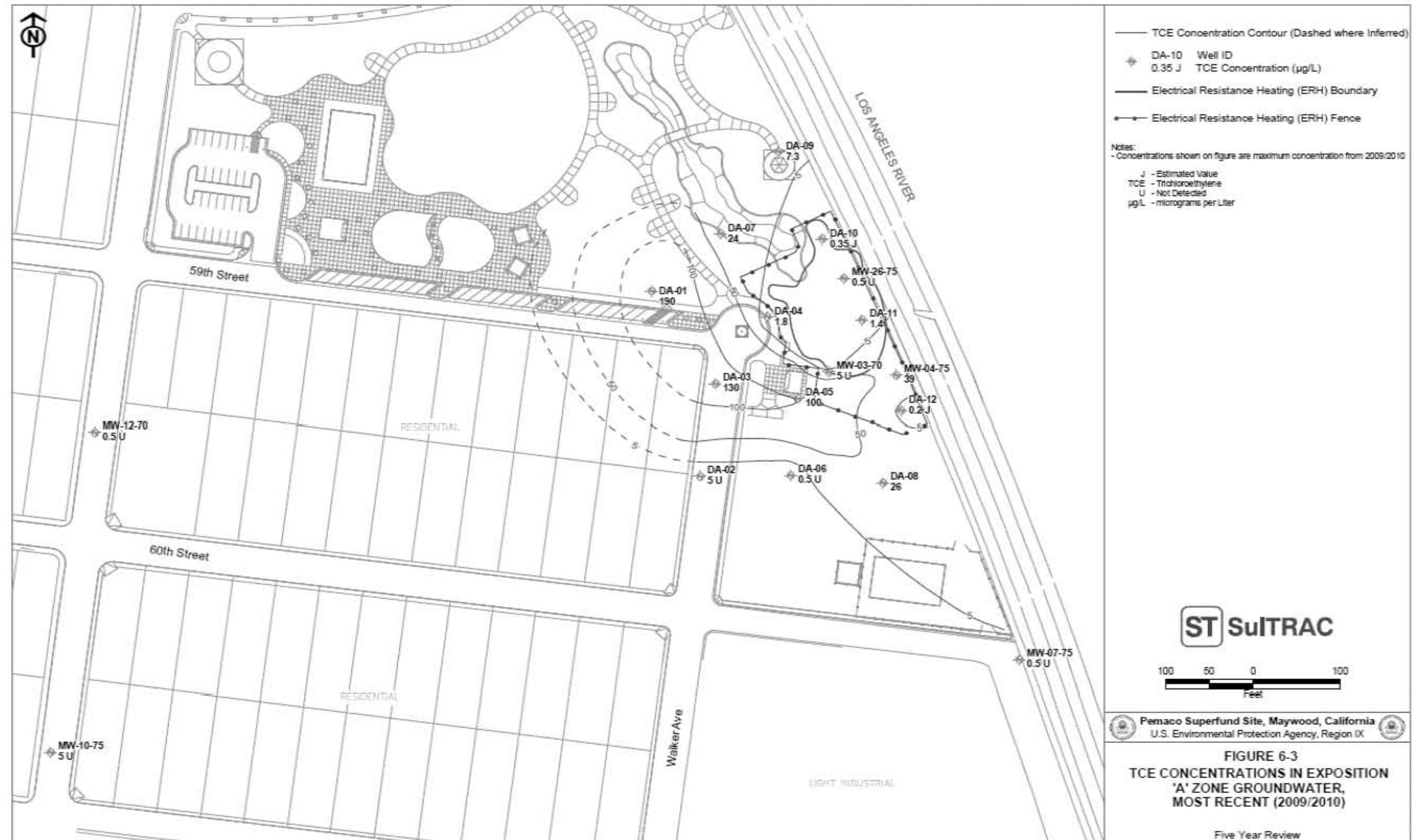
Figure 6-3 Post-ERH Maximum Concentrations of TCE in Exposition 'A' Zone Groundwater, Pemaco Superfund Site, Maywood CA
