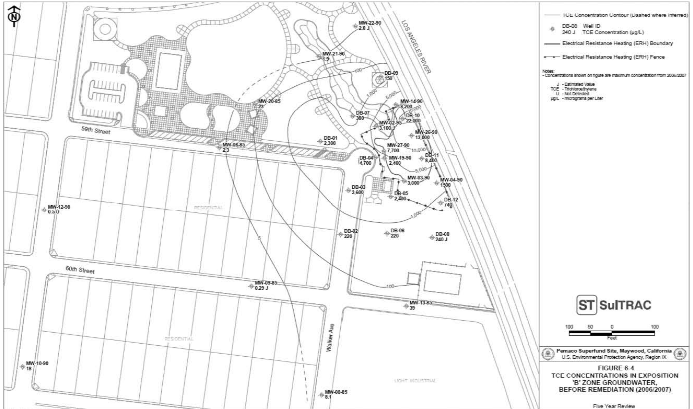
Figure 6-4 Pre-HVDPE Maximum Concentrations of TCE in Exposition 'B' Zone Groundwater, Pemaco Superfund Site, Maywood CA
