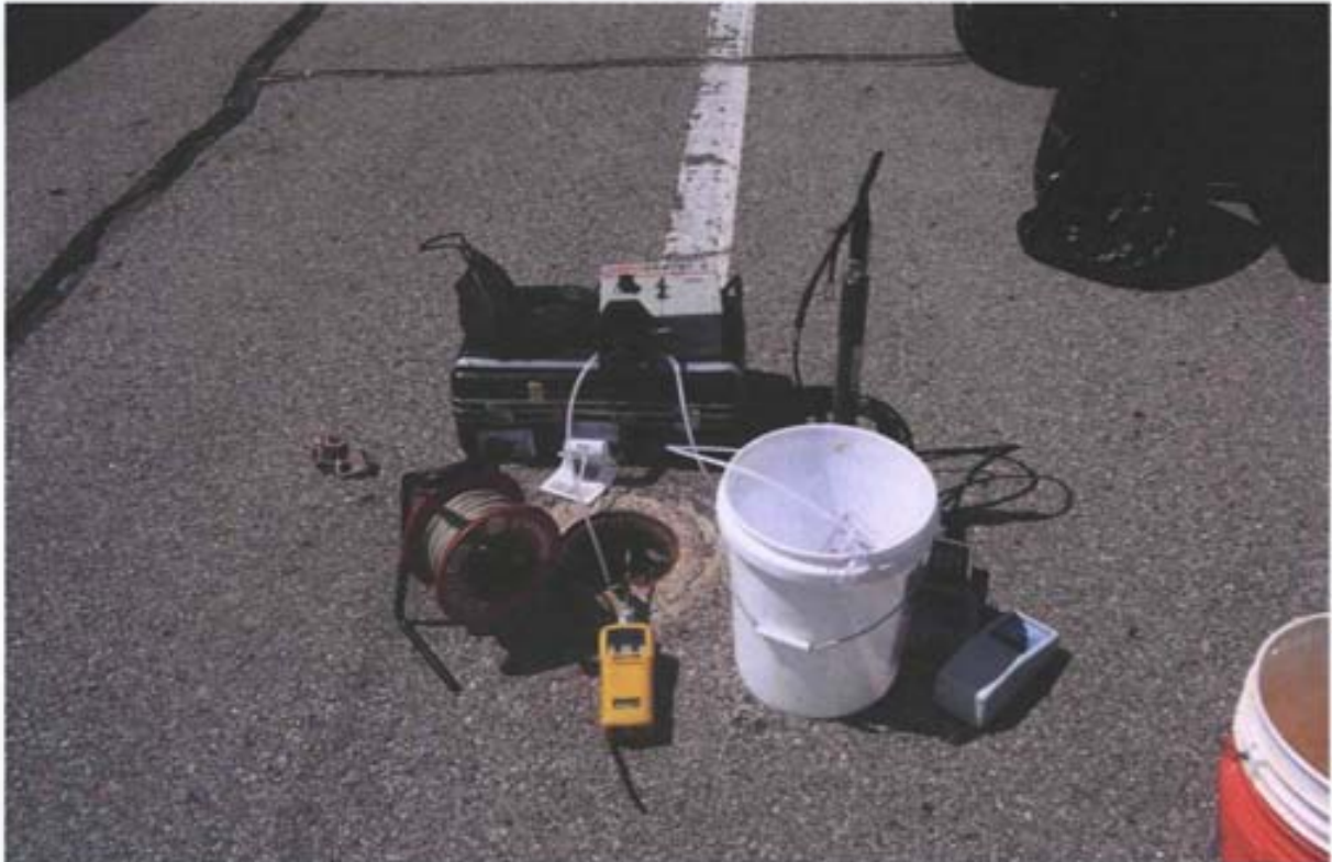
Photo 34: Close-up of low-flow sampling equipment at monitoring well SS30-MW-18 at Site SS-30.
