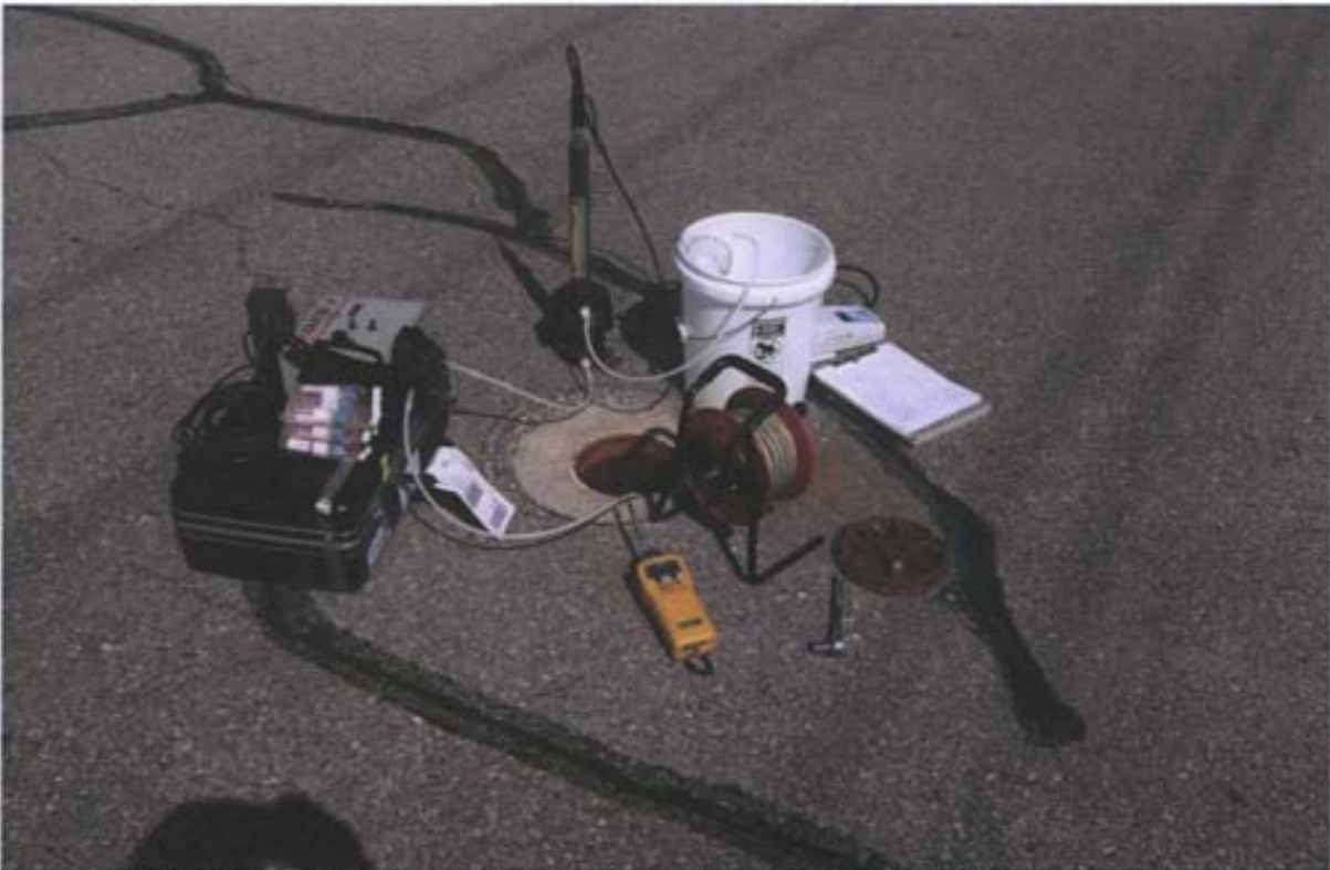
Photo 33: Close-up of low-flow sampling equipment at monitoring well SS30-MW-19 at Site SS-30.
