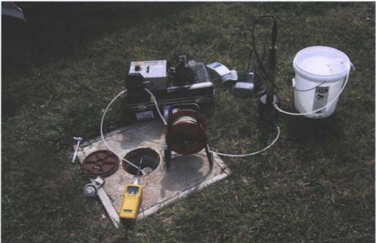
Photo 35: Close-up of low-flow sampling equipment at monitoring well SS30-MW-20 at Site SS-30.
