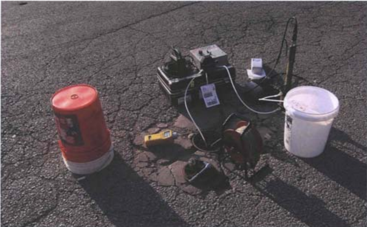
Photo 36: Close-up of low-flow sampling equipment at monitoring well SS30-MW-16 at Site SS-30.
