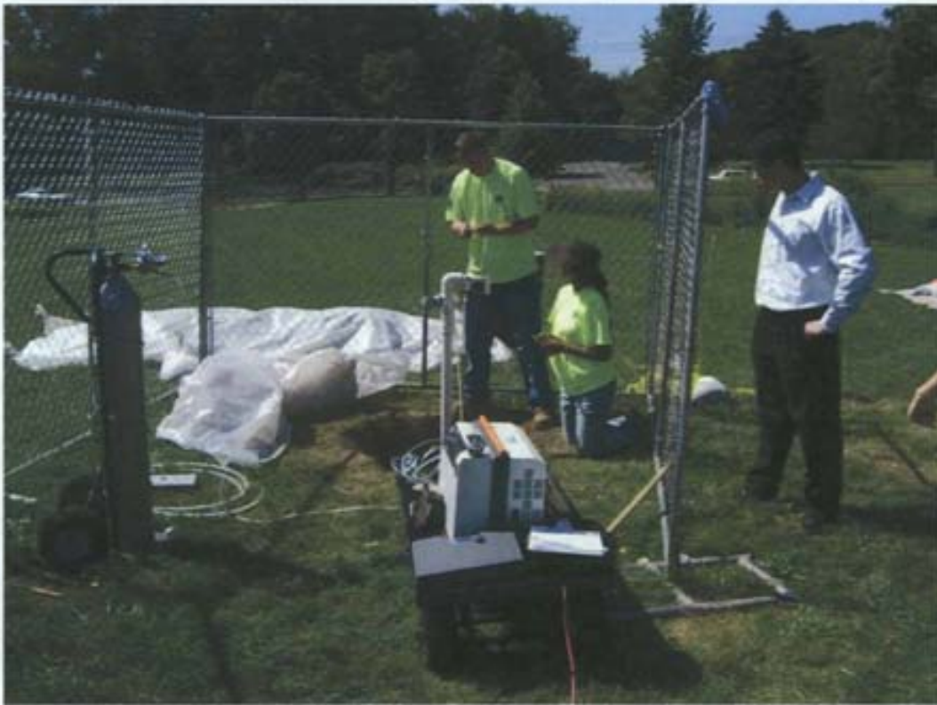
Photo Number 3 – August 2009: Injection point set up for Soil Gas Tracer Study
