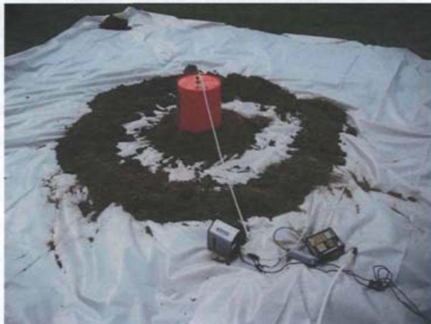
Photo Number 2 – August 2009: View of the soil gas probe set up for the Soil Gas Tracer Study.
