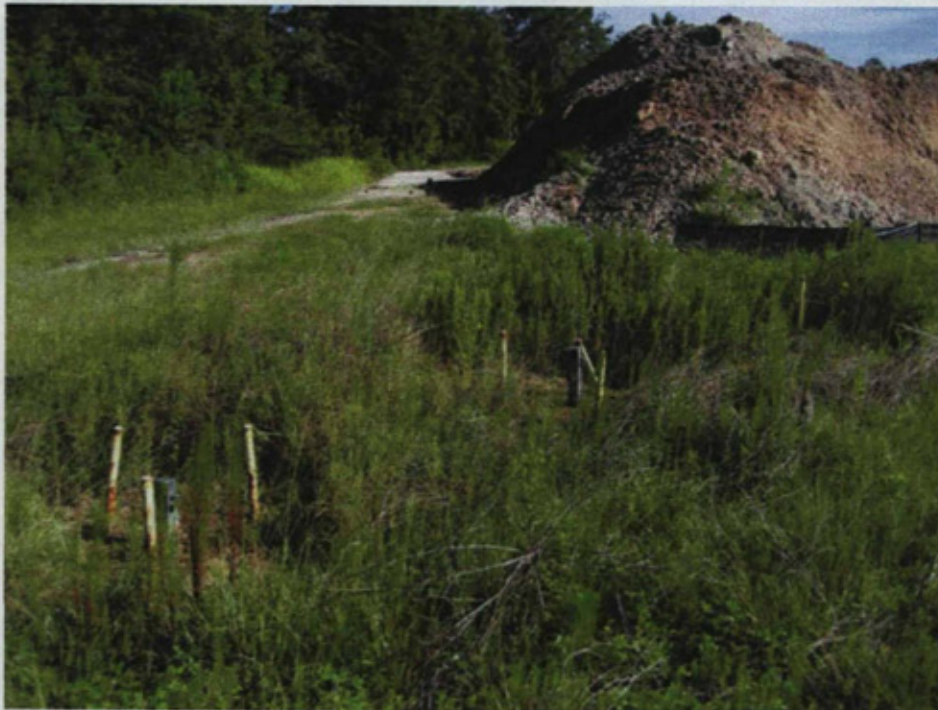
Monitoring wells showed elevated levels of PAHs and are located next to the mound of soil.
