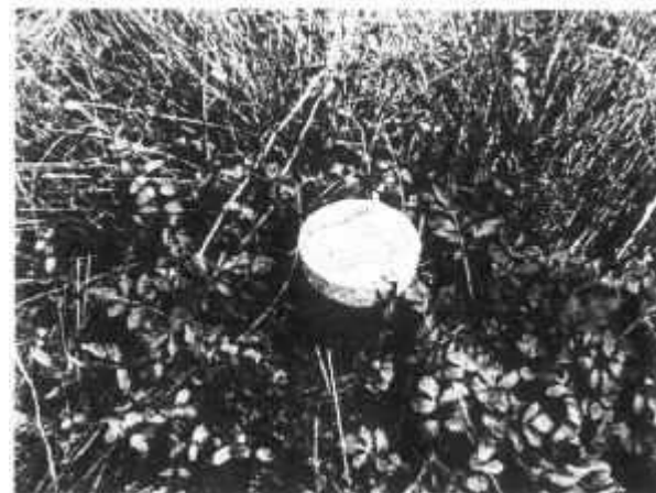
Old monitoring well - note missing lock.
