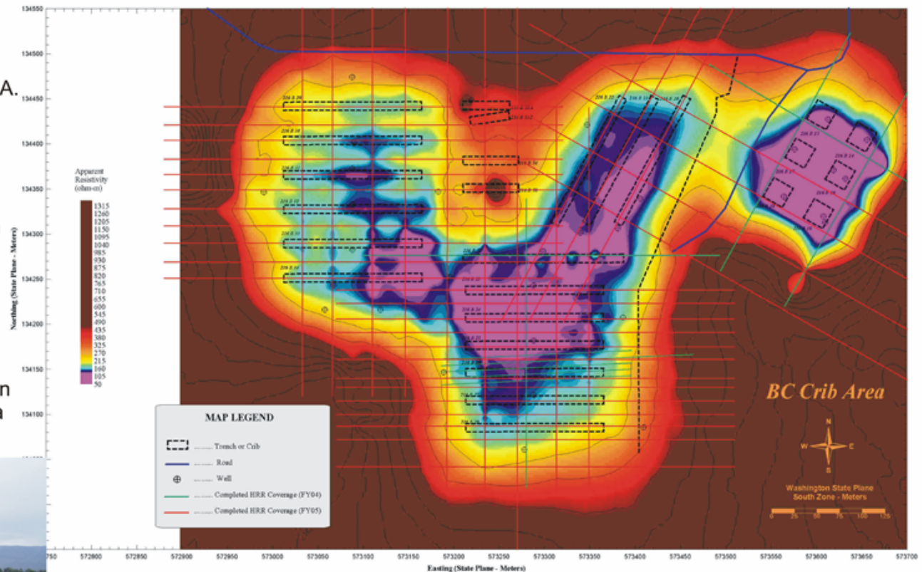
The map shows the apparent resistivity at a depth of 32 meter (105 ft).
