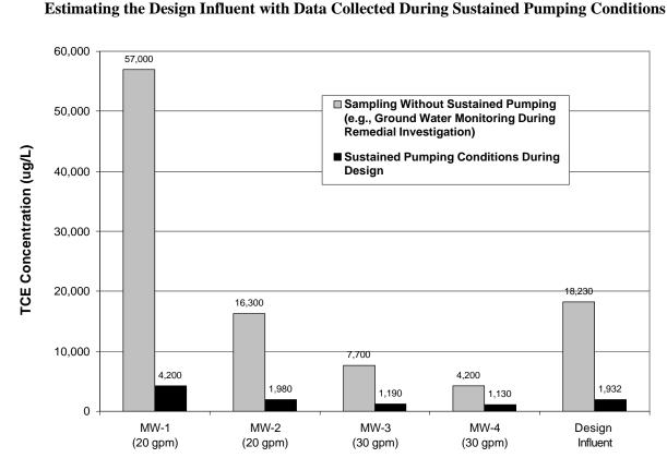
Expected Extraction Well Location Indicated by Nearby Monitoring Well (Expected Sustained Pumping Rate from each Extraction Well)
