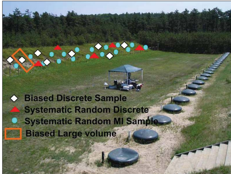
Figure 35. Schematic showing comparison of different sampling designs for a portion of a small arms range berm. Blue dots represent approximate locations where increments were collected to build MI sample. White and red symbols represent approximate locations of discrete samples.
