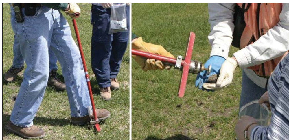
Figure 27. Coring tool designed specifically for collecting cohesive multi-increment soil samples.
