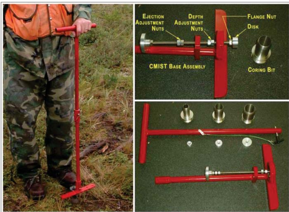
Figure C-1. CRREL Coring Device (CRREL 2004a; CRREL 2009). Note various size coring shoes. Increment cores from a single Sampling unit should be of the same size
