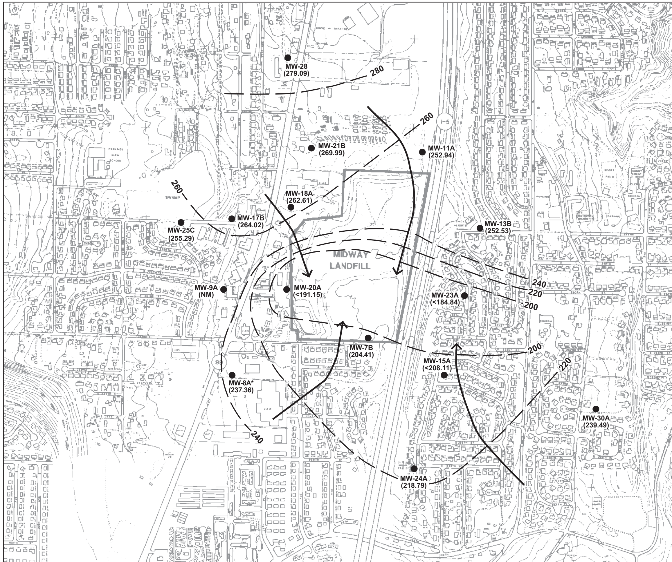
Figure 3 Generalized Sand Aquifer Potentiometric Surface Map, October 2008 Midway Landfill Kent, Washington
