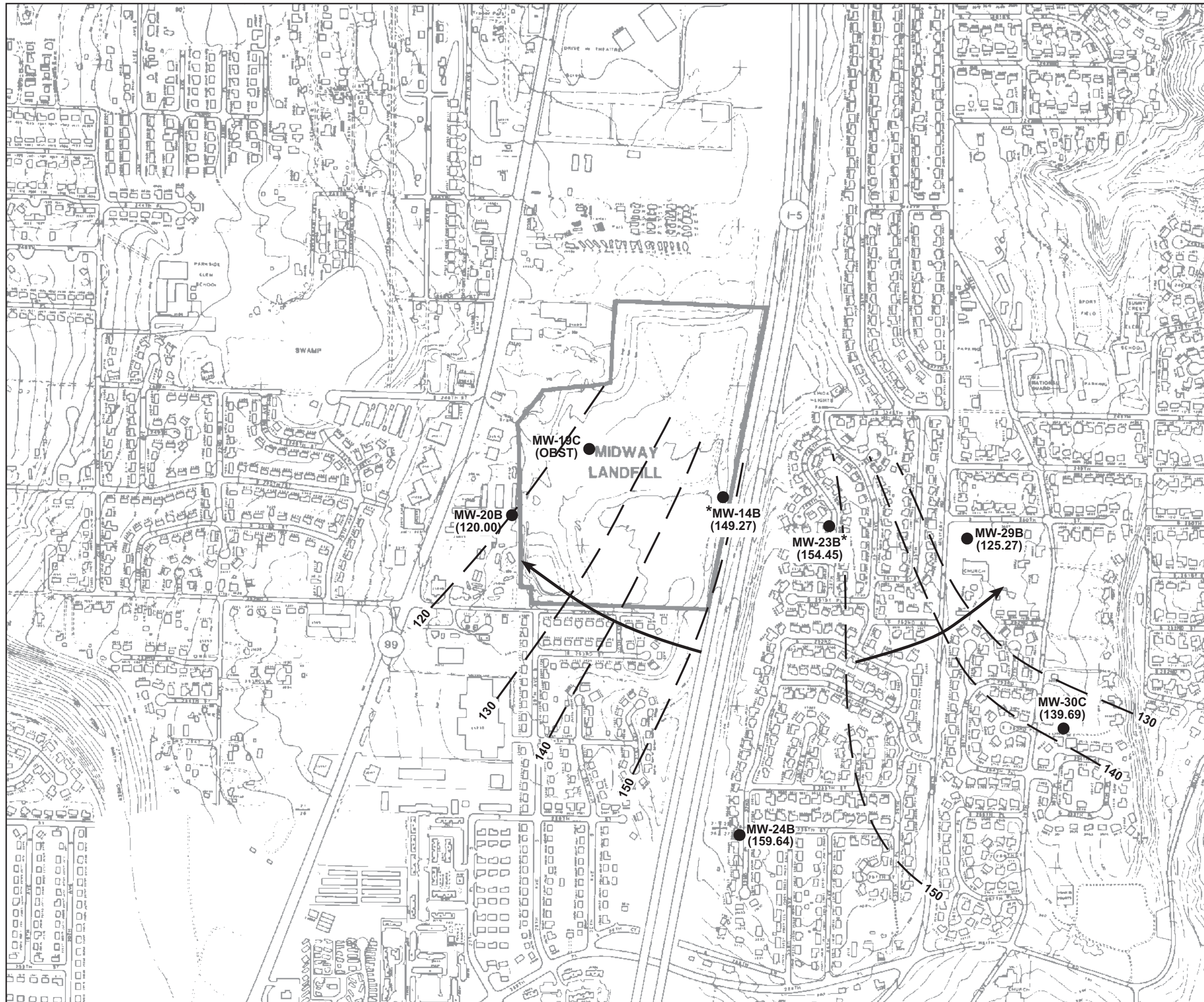
Figure 4 Generalized Southern Gravel Aquifer Potentiometric Surface Map October 2008 Midway Landfill Kent, Washington
