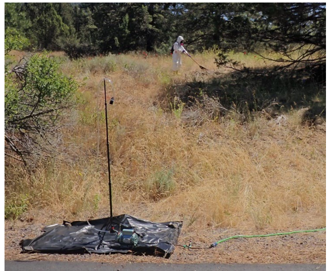
Figure 3: Activity-based sampling took place in 2023 to evaluate potential risk from airborne asbestos fibers.
