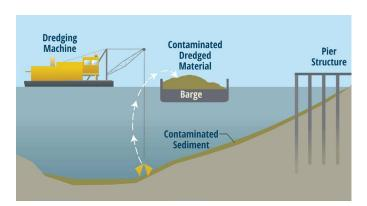
**Dredging** removes contaminated sediment from the waterway. After removal, dredged material will be disposed of in a permitted landfill.
