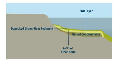
**Enhanced Natural Recovery** uses a thin layer of sand to cover the contamination and speed up the natural recovery process.
