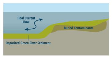
Monitored Natural Recovery relies on the natural flow of cleaner sediments from upriver to cover contaminated sediments in the waterway. The clean sediments are monitored to measure the reduction in contamination over time.
