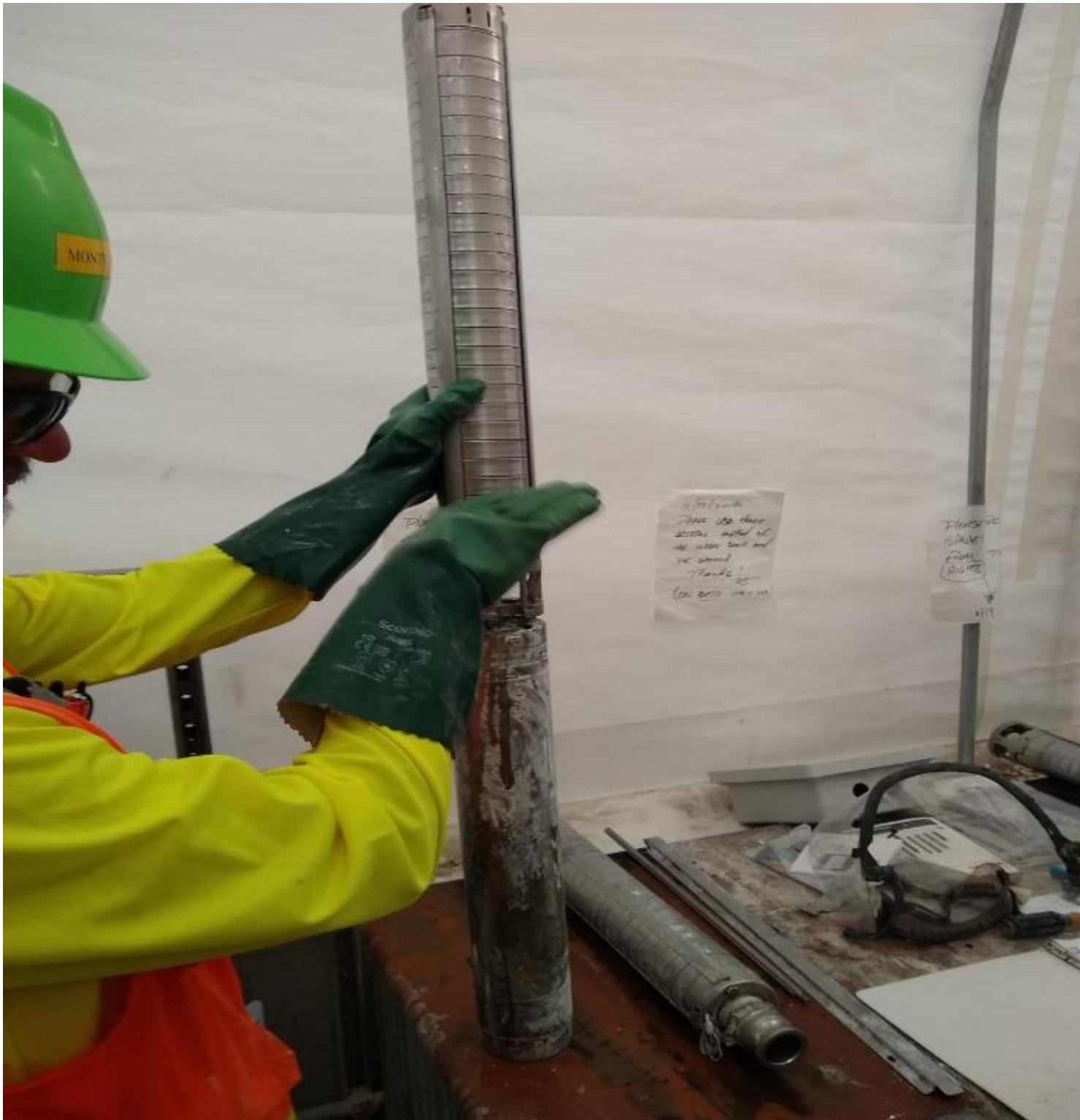
Photograph 10 - IMG_20200722_092754060: Former Well #423 Treatment Facility; explanation of well 423 pump operation, bottom half is motor middle area is well screen
