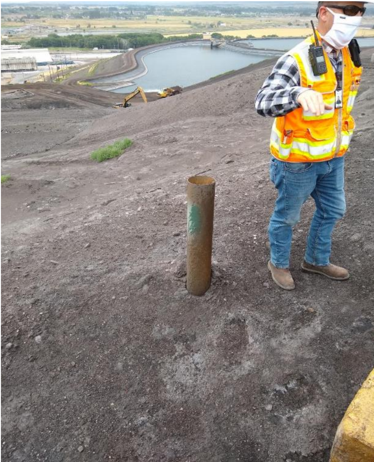
Photograph 29 - IMG_20200722_110920856: Gypsum Stack; vertical piezometer, measures seepage through the liner
