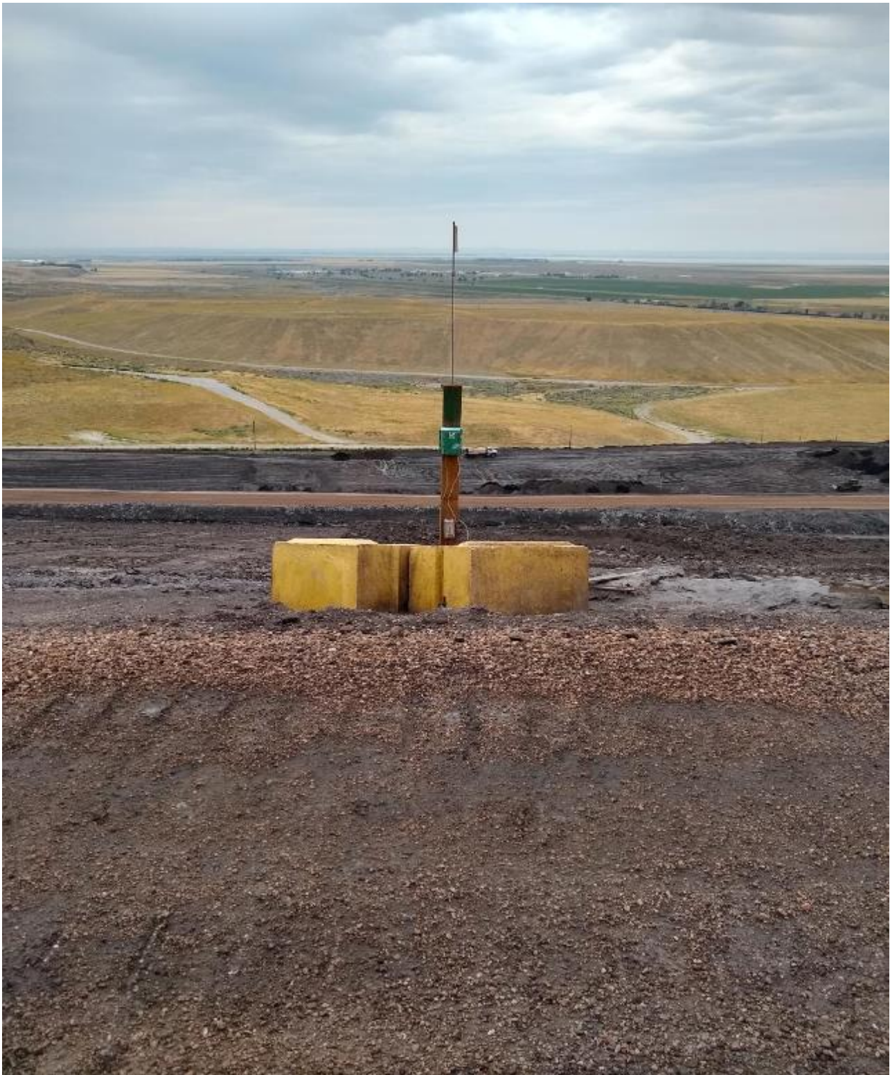
Photograph 25 - IMG_20200722_105512907_HDR: Gypsum Stack; lateral piezometer, measures water under the liner
