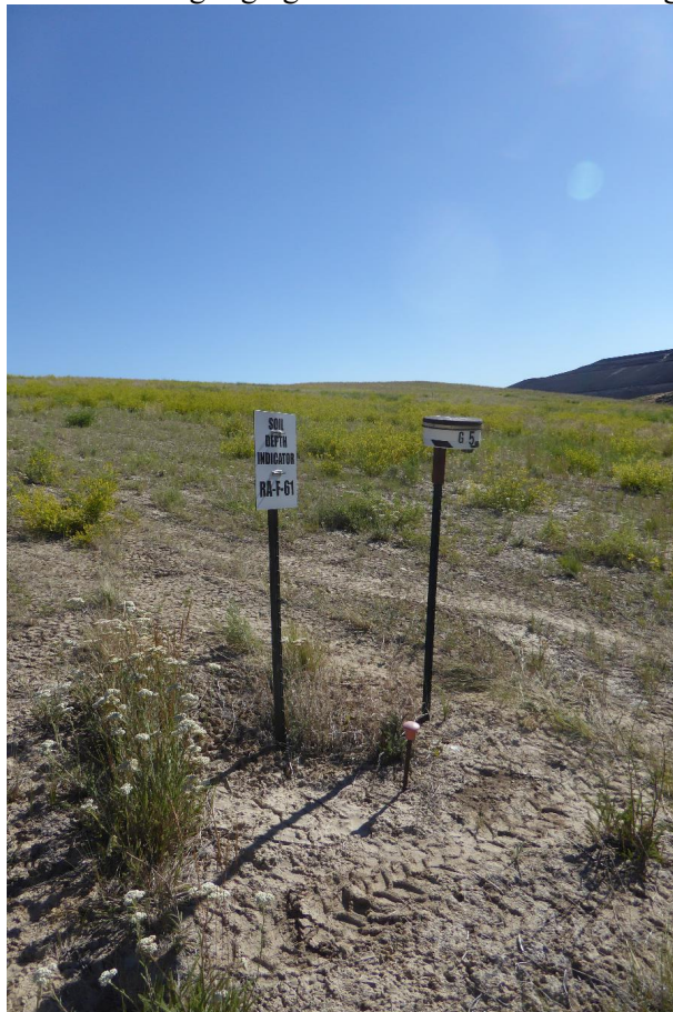
Soil depth indicator on top of RA-F on FMC OU
