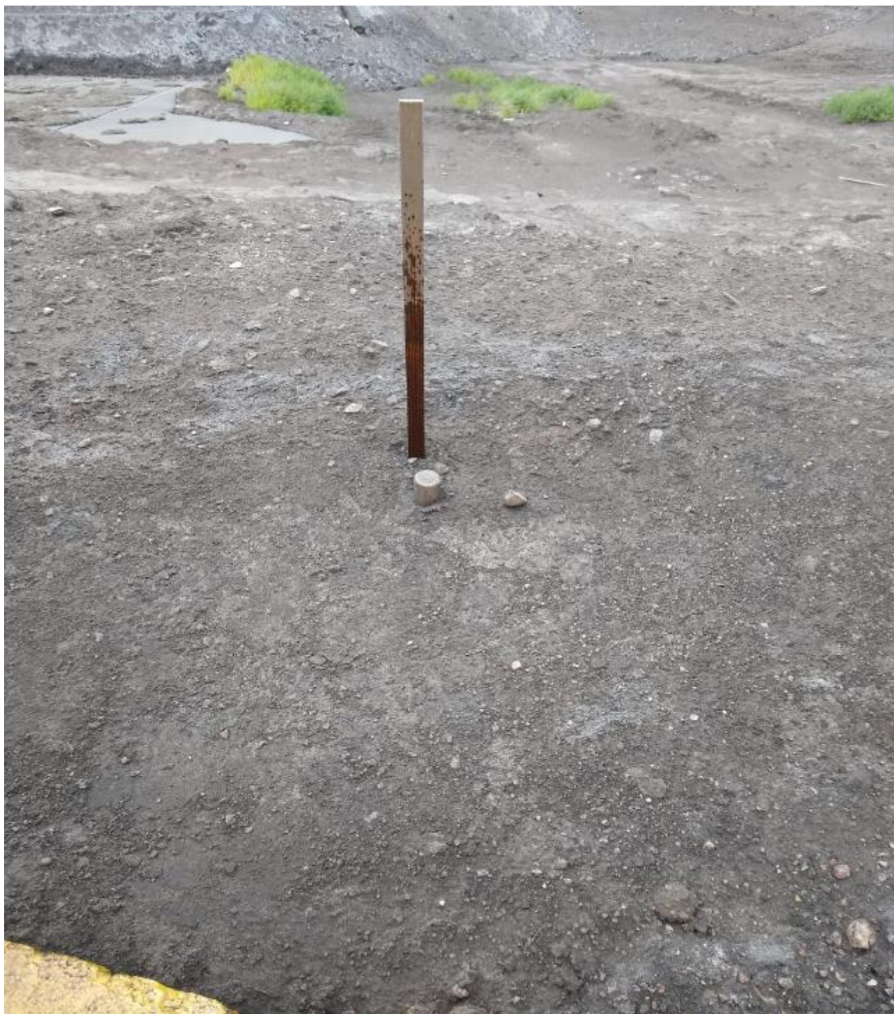
Photograph 28 - IMG_20200722_110802997: Gypsum Stack; survey monument for settlement measurement
