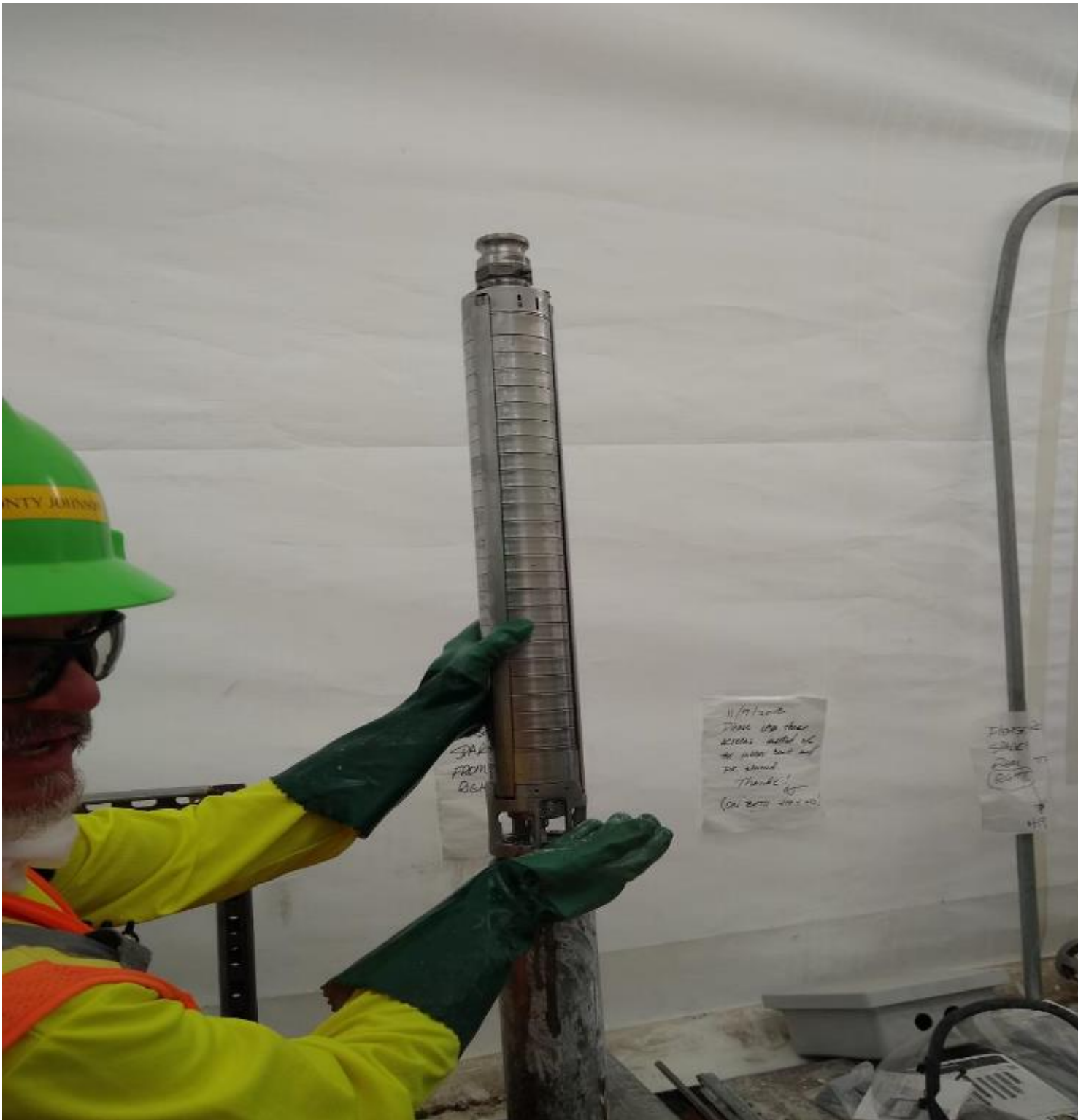
Photograph 9 - IMG_20200722_092750527: Former Well #423 Treatment Facility; explanation of well 423 pump operation, bottom half is motor, middle area is well screen
