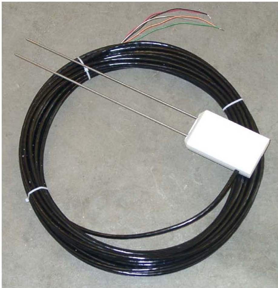
Figure 8-5. TDR Probe and Coaxial Cable.
