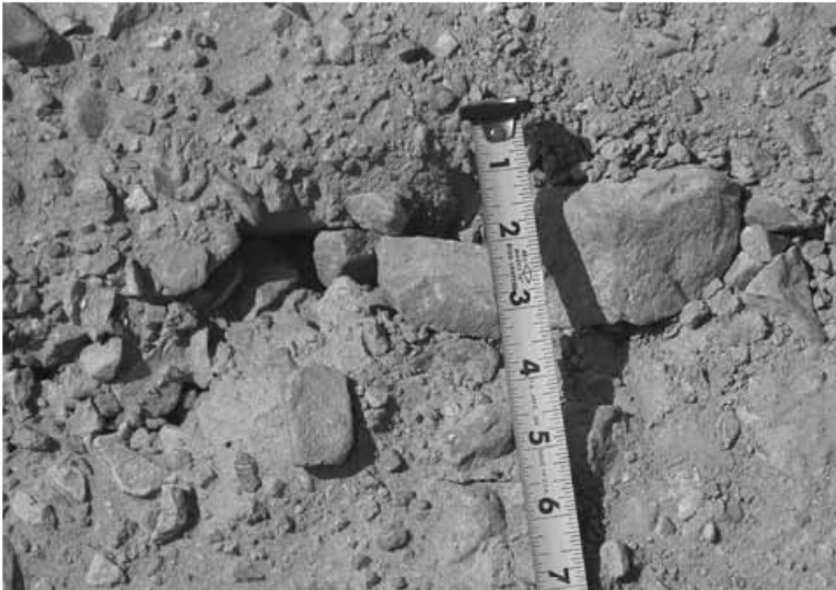
Figure 7-16. Surface Tension Cracks in Cover Soils from Differential Settlement of Underlying MSW.
