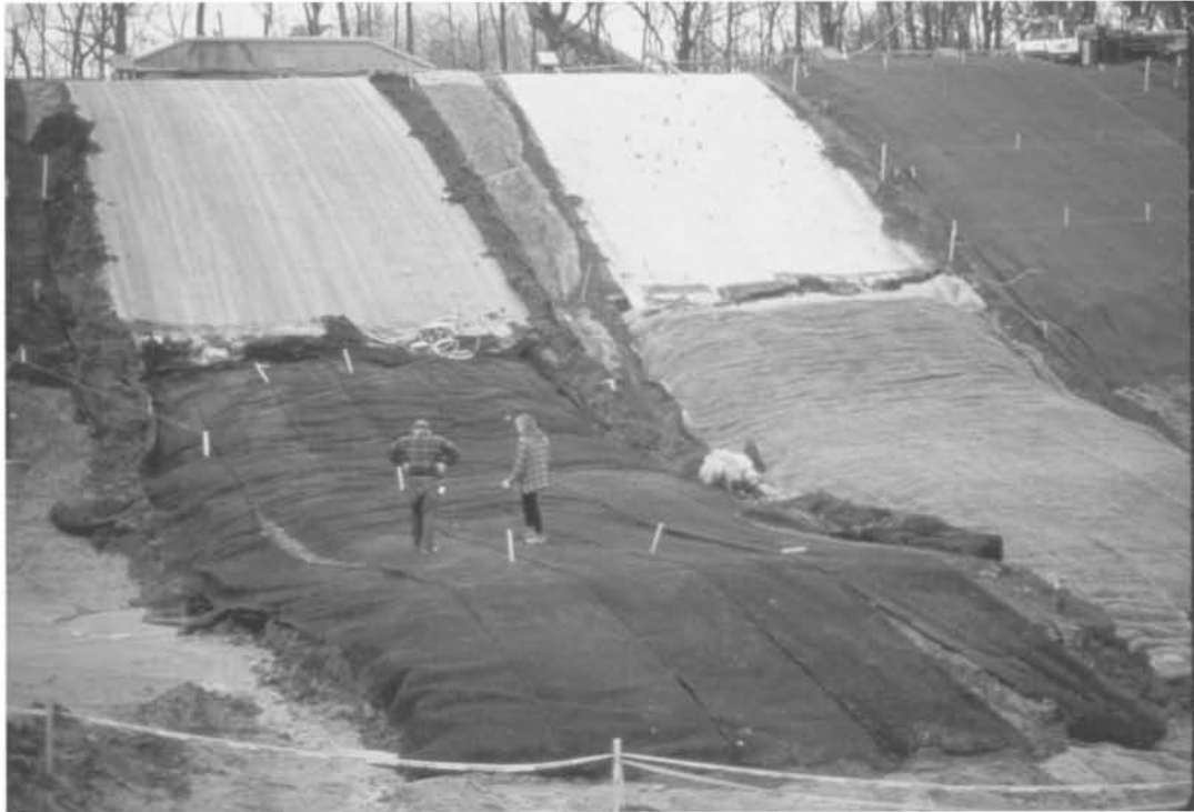
Figure 7-15. Plots G (Left) and H (Right) Approximately Two Months After Construction and Several Days after the Slide in Plot G.
