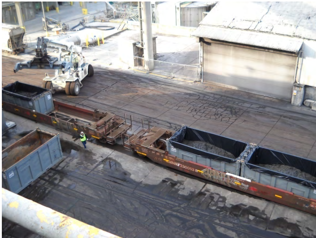
Photograph 3-7. Transloading from Vault to Containers (November 9, 2011)
