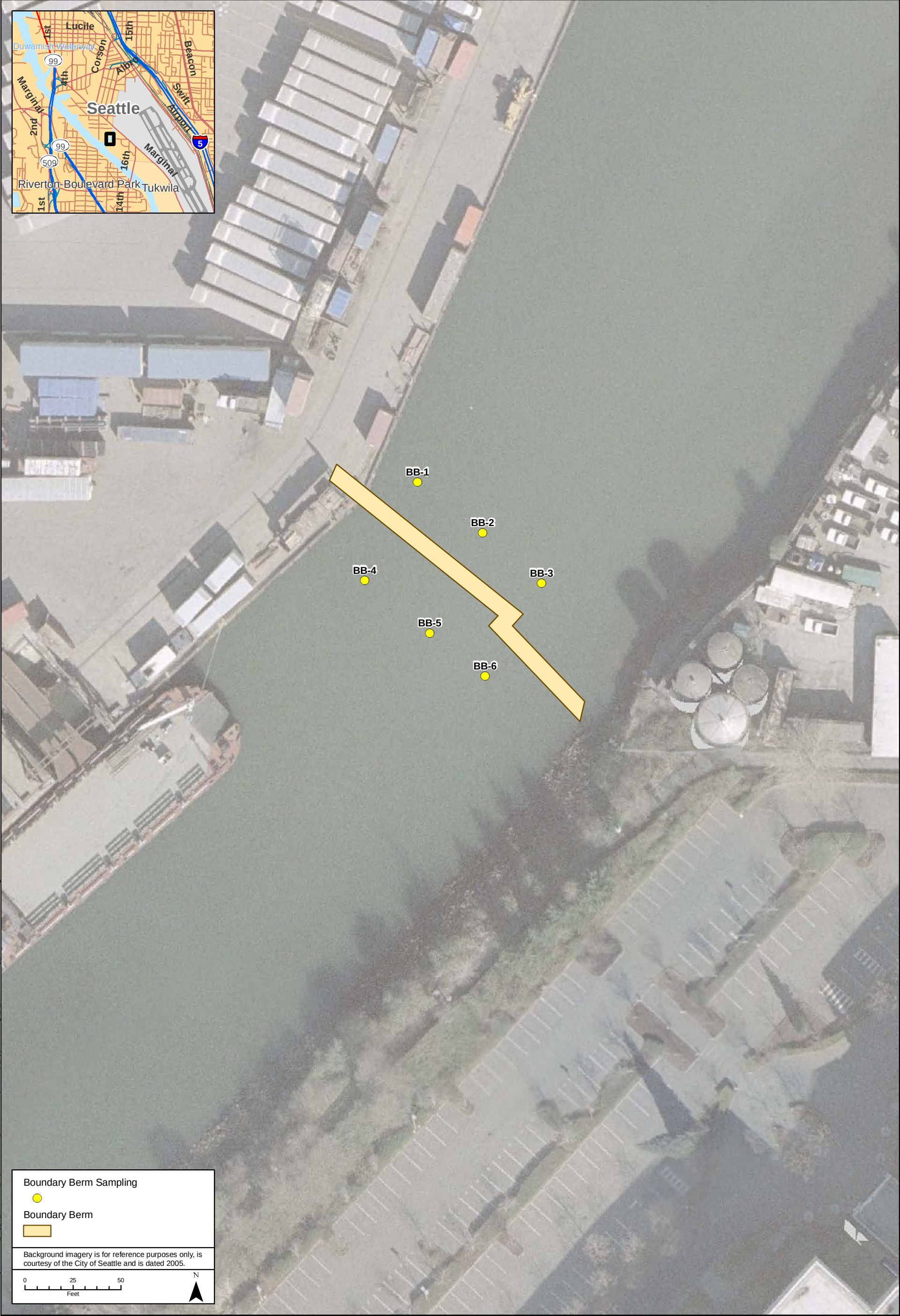
Figure 3-3. Boundary Berm Turbidity Sampling Slip 4 Removal Action
