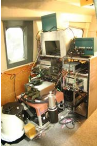
Image A2: View of chemical sensors: high speed infrared spectrometer, lower left corner; infrared line scanner is out of view behind the line scanner.
