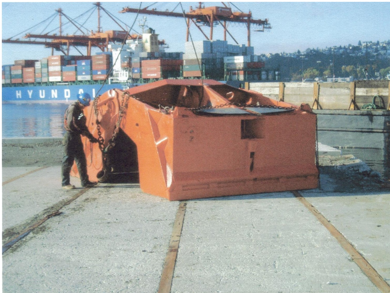
FIGURE 5-1 Environmental Dredge Bucket Used at Todd Shipyard, Harbor Island, Washington
