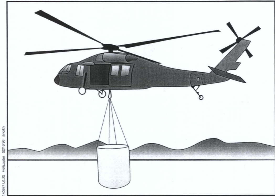
Figure 5-2 Blackhawk Helicopter Application of Cap-and-Fill Material OU-C Record of Decision
