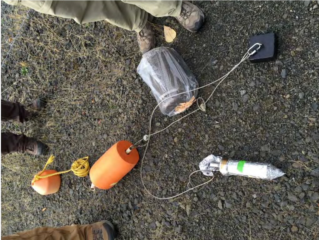
Photograph 6 – Typical setup for surface water sampling equipment during 2015 sediment cap performance monitoring.
