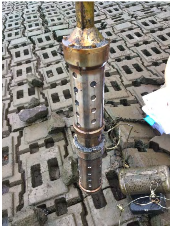
Photograph 7 – Recovered sub-armor, inter-armor, and surface water sampler from early warning sample location number 12 during September 2015 sediment cap performance monitoring.
