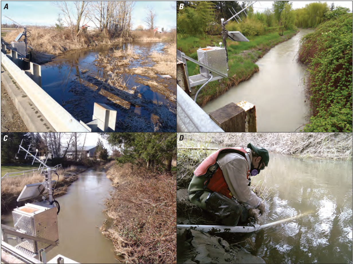
Figure 6. U.S. Geological Survey streamflow-gaging stations and turbidity sensor installation on the Sumas River, Whatcom County, Washington, 2011–13. (A) Sumas River at Massey Road near Nooksack (12214300), February 1, 2011; (B) Sumas River at South Pass Road at Nooksack (12214350), May 11, 2011; (C) Sumas River near Sumas (12214500), February 1, 2011; and (D) turbidity sensor installation, April 20, 2011. Photographs by Steve Sumioka, U.S. Geological Survey.
