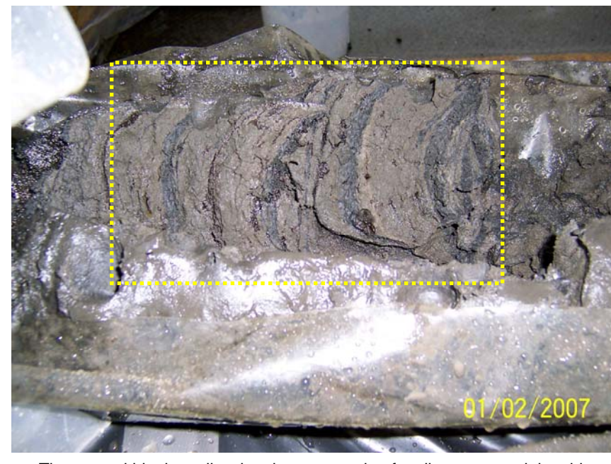
The area within the yellow box is an example of sediments containing thin layers of tar. Note the scale is not clear from picture. If any layers are more than 2-inches thick, then this would meet the definition of substantial product.
