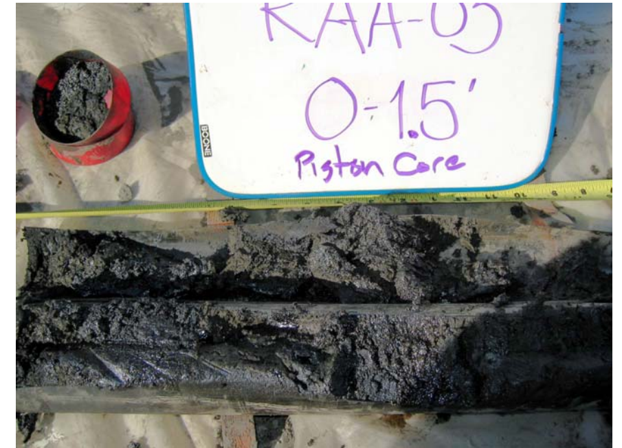
Sediments containing bands of tar and semi-solid product greater than 2 inches
