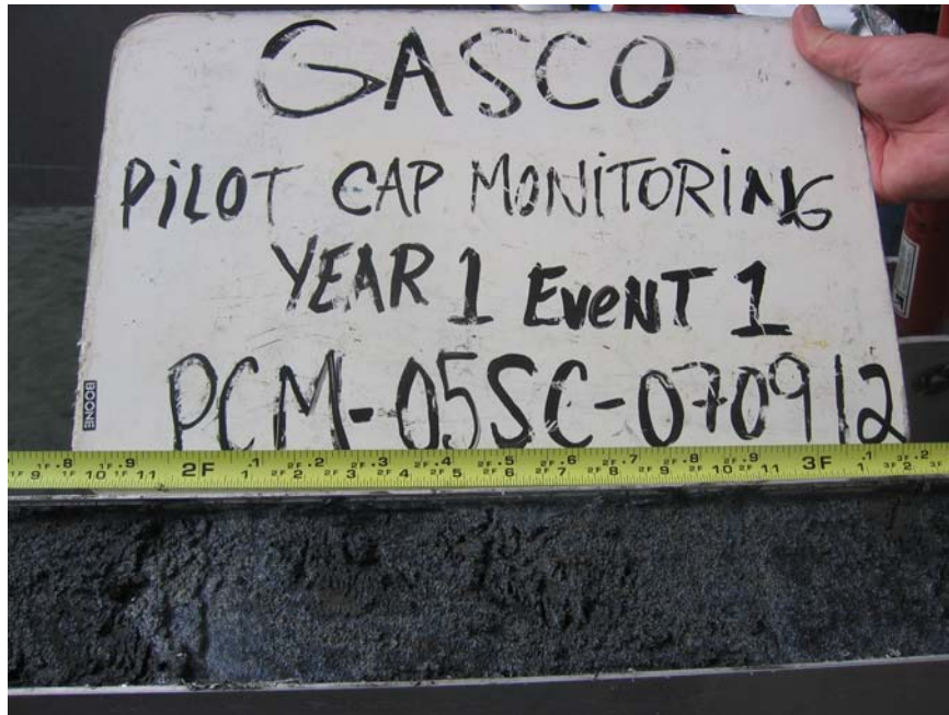
Sediments saturated with product over a several inch interval
