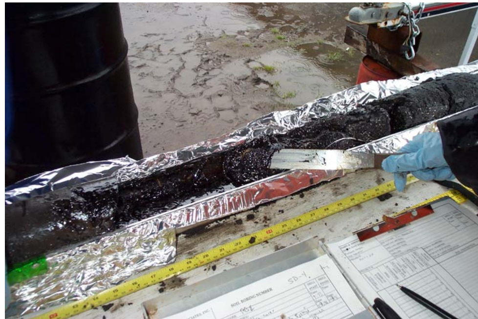
Sediments with substantial tar and pockets of mobile liquid product
