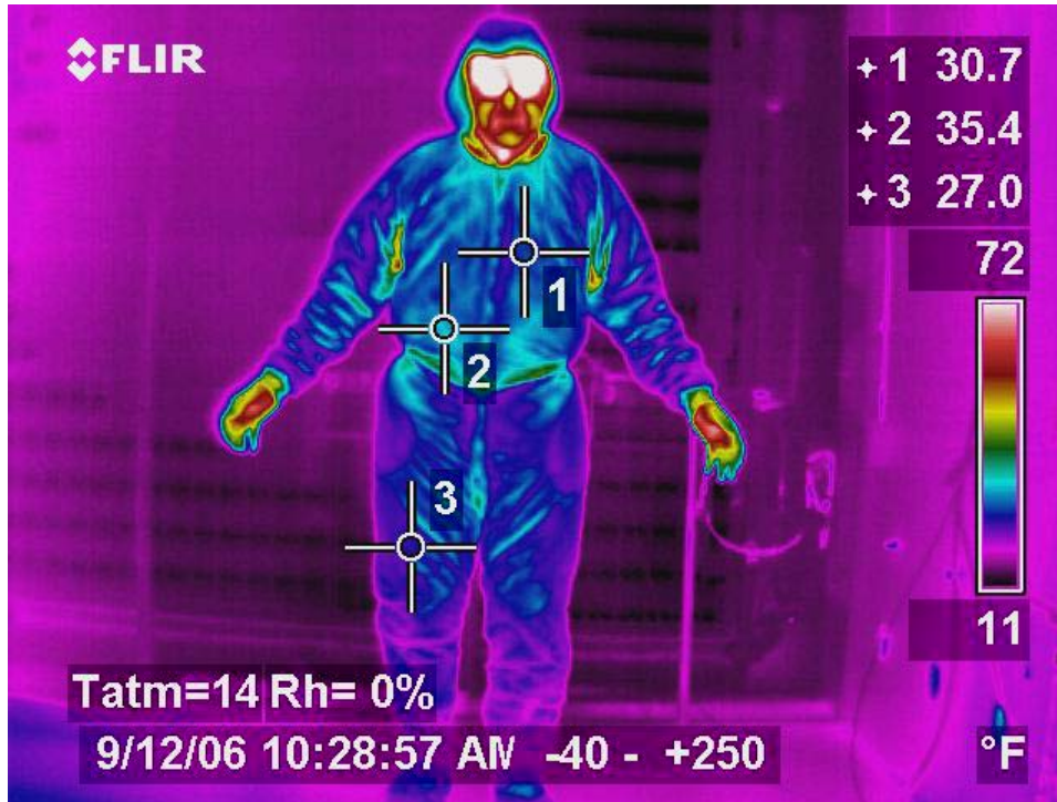
Figure 5. Frontal view of 400-weight Thinsulate garment. Typical surface temperatures 27-35°F.
