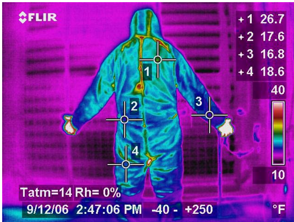
Figure 6. Back view of aerogel garment. Typical surface temperatures 17-27°F.
