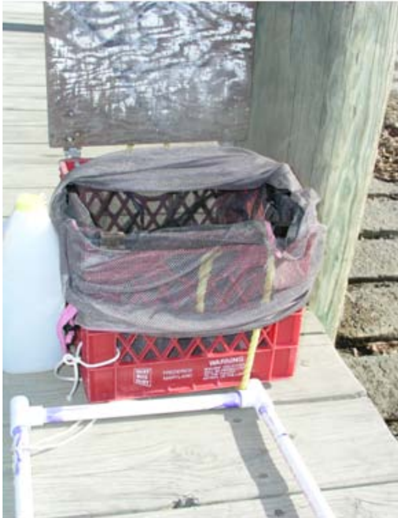
Figure 2. Oyster sampling apparatus used in the Magothy River Association along with mesh liner used to collect benthic macroinvertebrates. The oyster sampling apparatus was adapted from the Magothy River Association protocol which samples viability of the oyster reefs in the Magothy River. A mesh lining was inserted to collect macroinvertebrates while excavating dredged shell substrate along with live oysters. The quadrat used was 29 cm x 29 cm x 35 cm.
