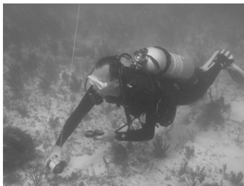
Figure 3. Image of Diver A following a compass heading during a transect. A diver reel leads to the GPS unit at the surface.
