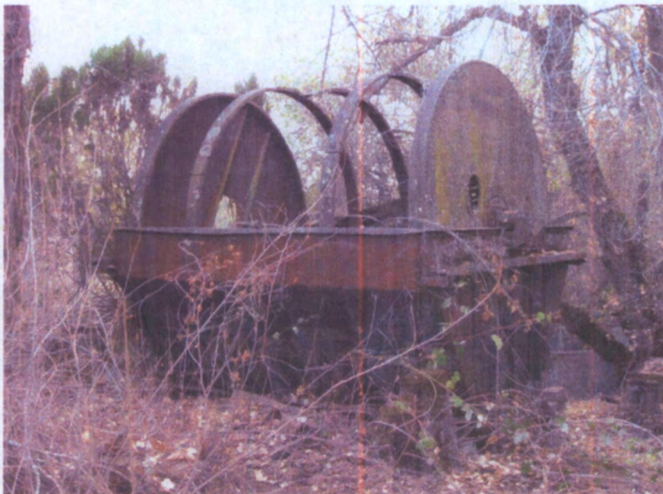
View of coal tar tumbling box located at the former Amador Metals Reduction (Cyanide) Plant used to coat the ore prior to cyanidation
