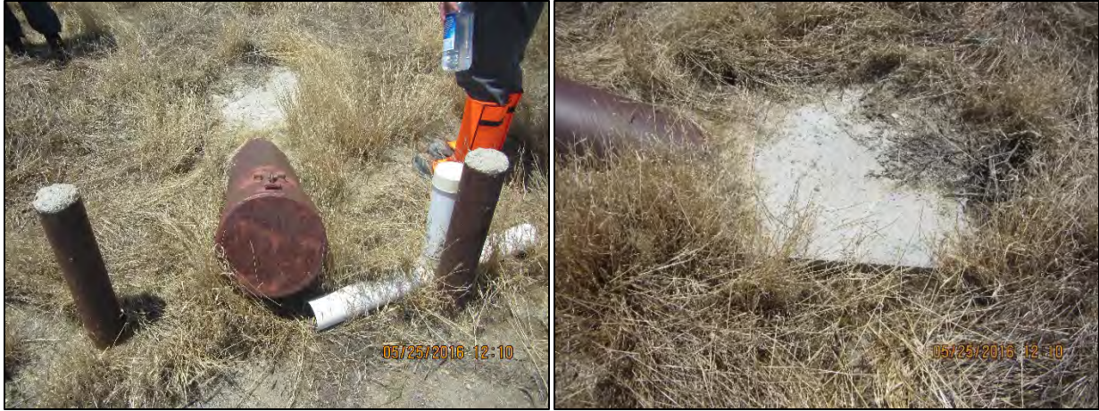
Photo 27. Neutron Probe Tube at City OU Landfill and Holes near Footings.
