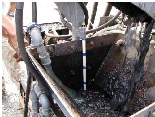
Figure 6-5. Iron guar mixture prepared for direct injection.
