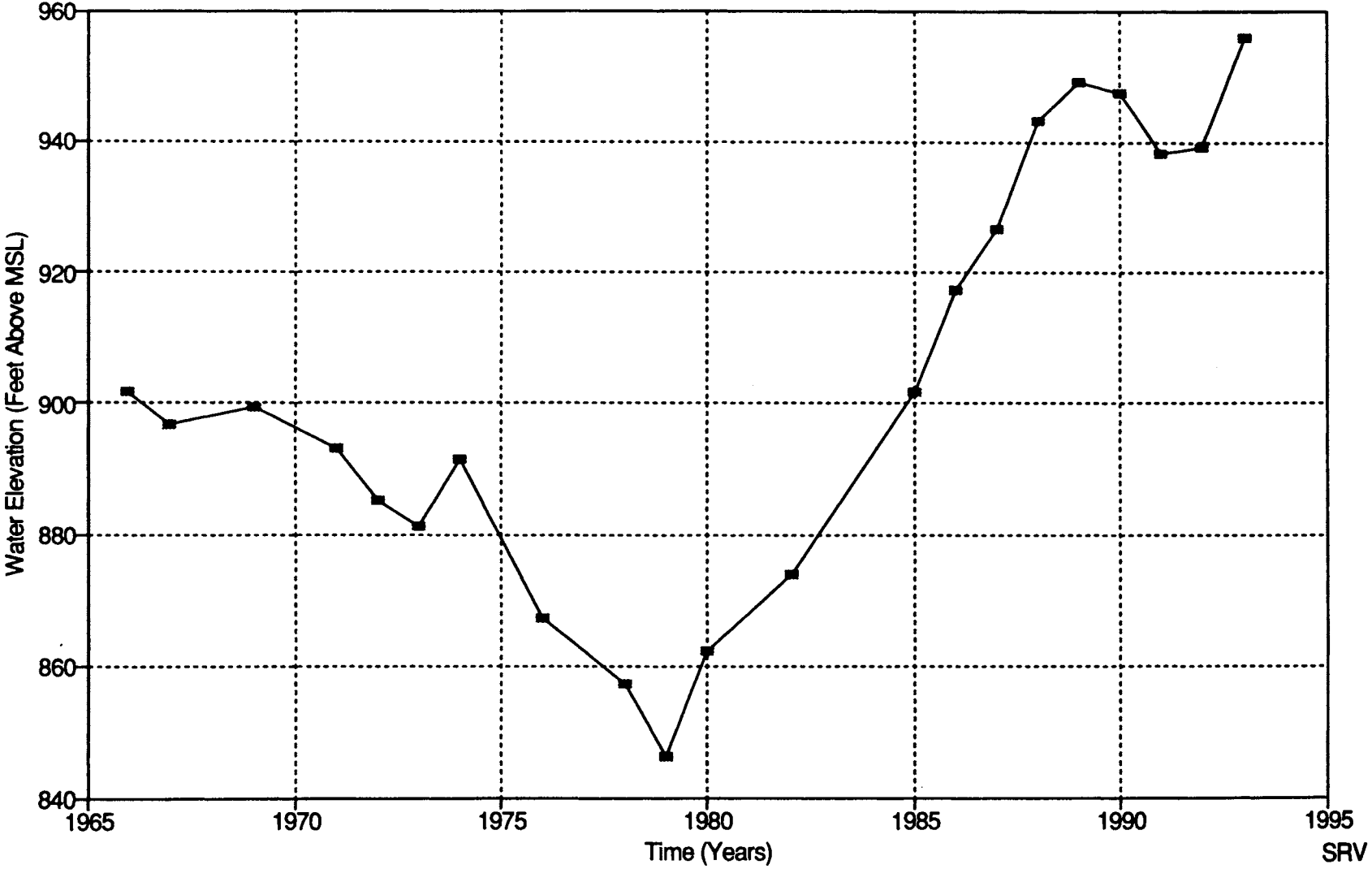
Hydrograph: Middle Alluvial Unit Aquifer Well: A-01-06 14AAA2
