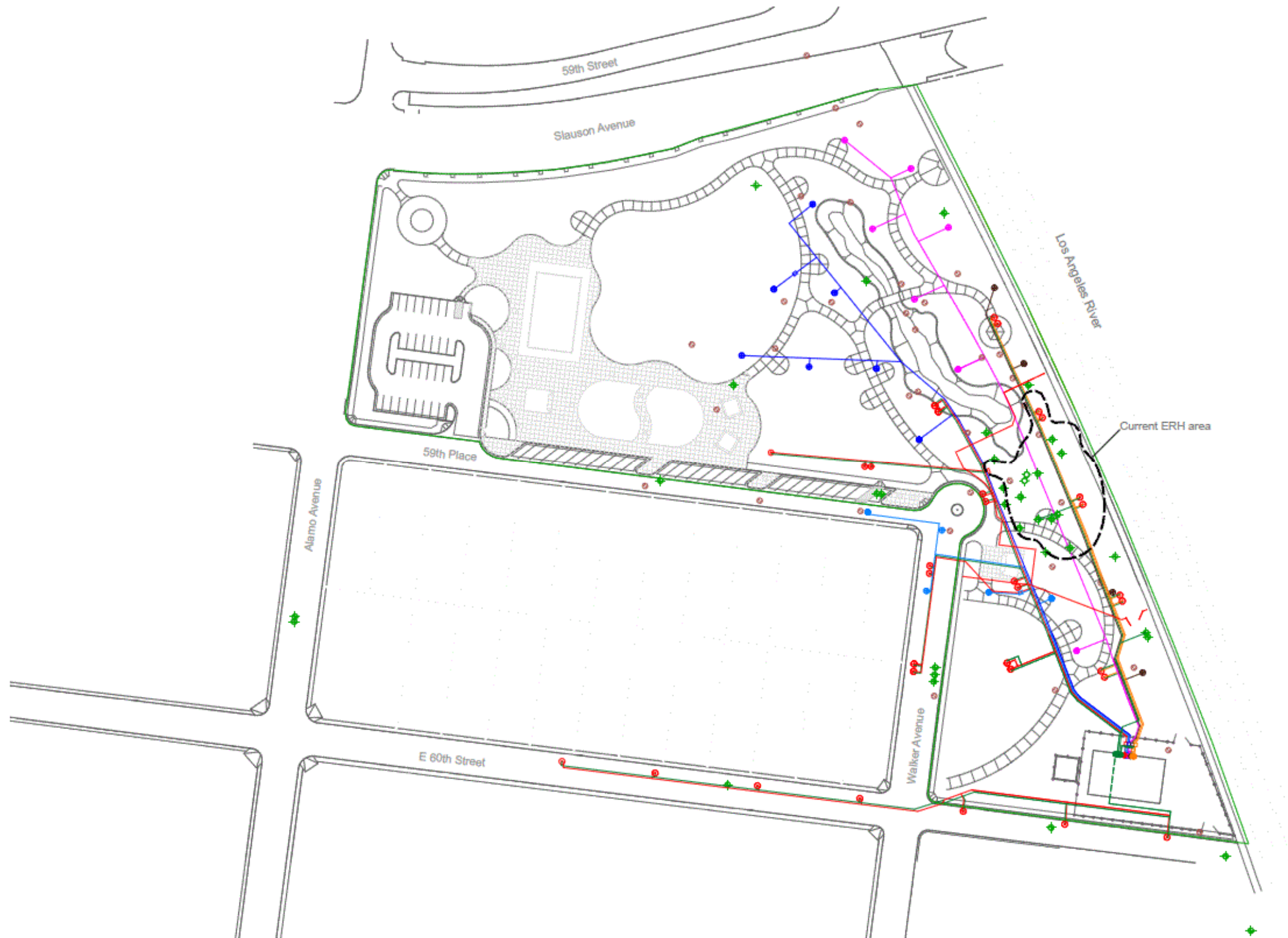
Figure 4-1: Pemaco Site Groundwater and Vapor Extraction System
