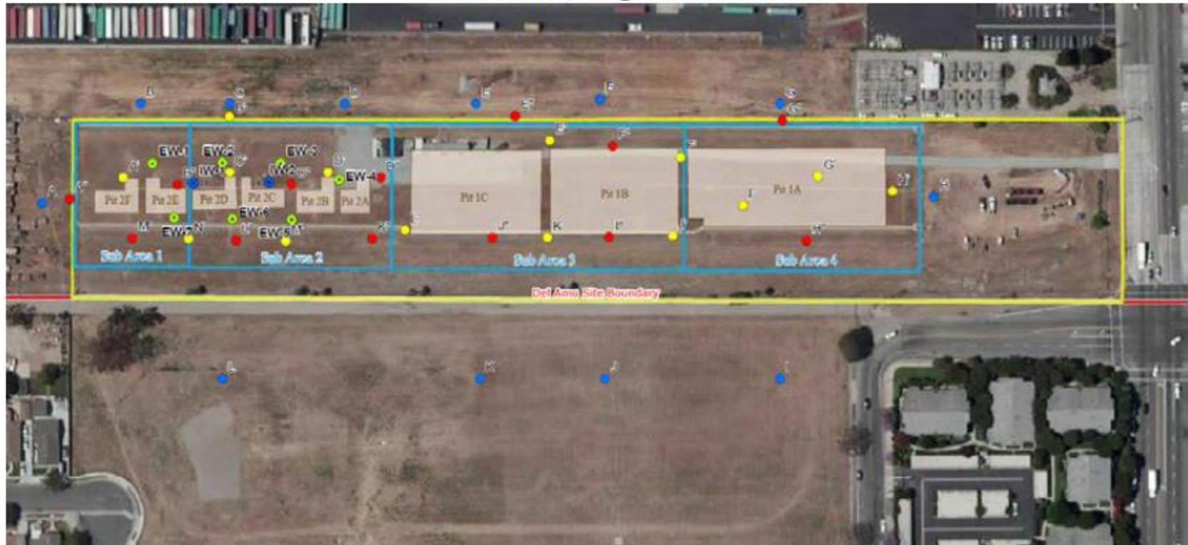
Former Pits, Cap, SVE-IBT System, and Monitoring Wells
