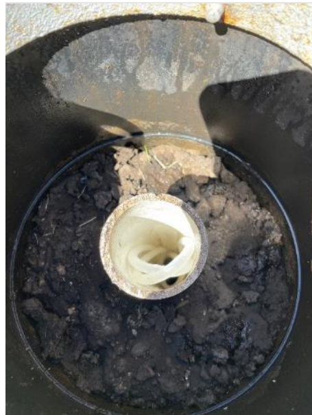
MW 165A with protective casing cover removed. The plug was not locked.
