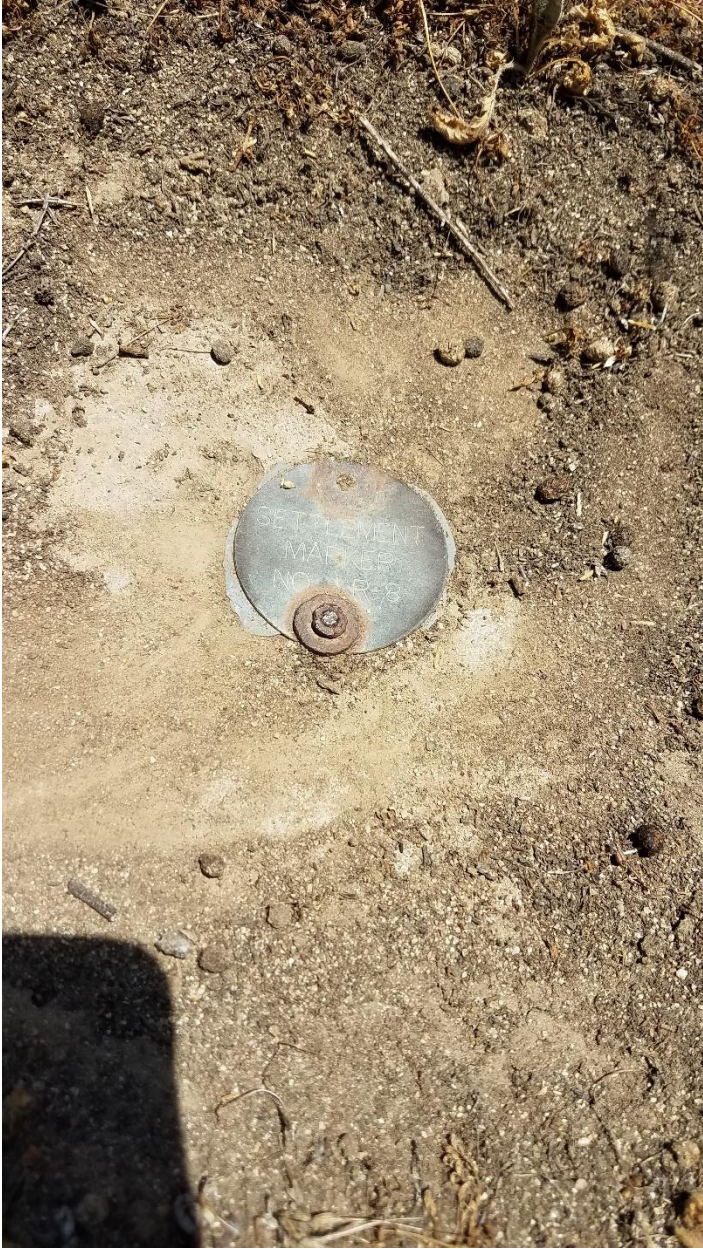
Settlement monument in Ramparts sump area
