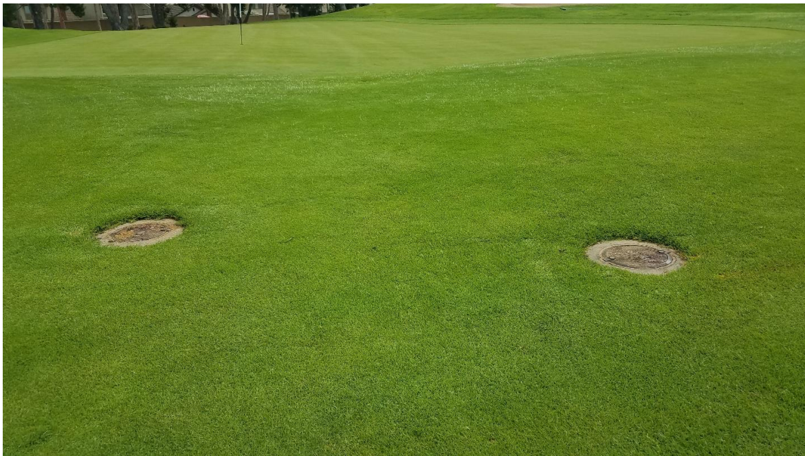
Well monuments in good condition on site; P-3D, P-3S
