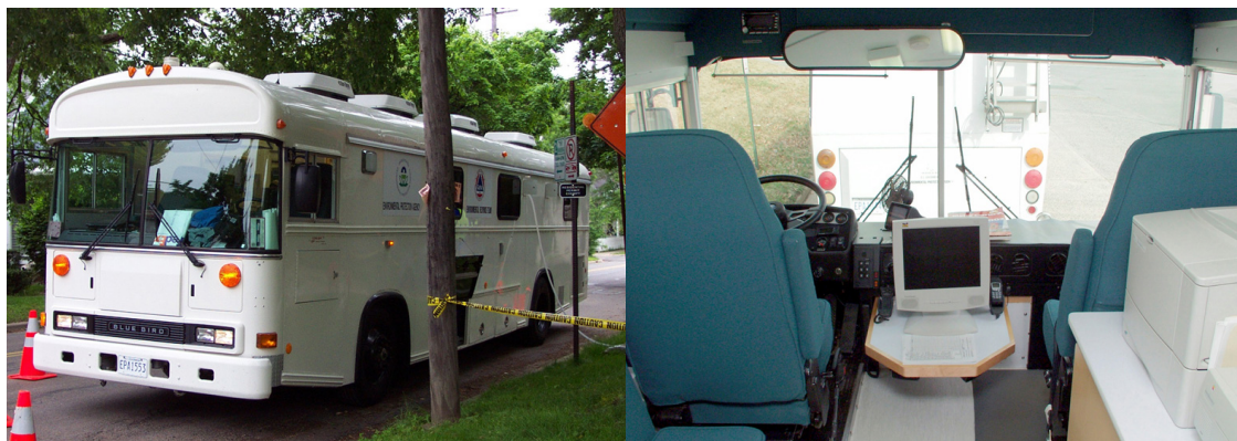
EPA used a Trace Atmospheric Gas Analyzer (TAGA) mobile laboratory during the vapor intrusion investigations to test for contaminants in indoor and outdoor air. These images show the exterior and interior of a TAGA mobile laboratory.
