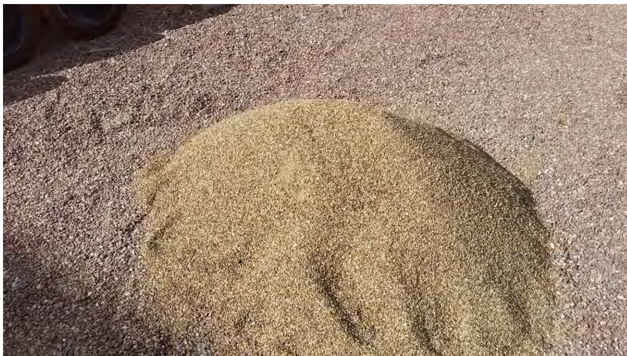
Gravel removed from TARP AOP treatment trains presumed to be coming from the piping system due to the past failure of the R-009A well screen.
