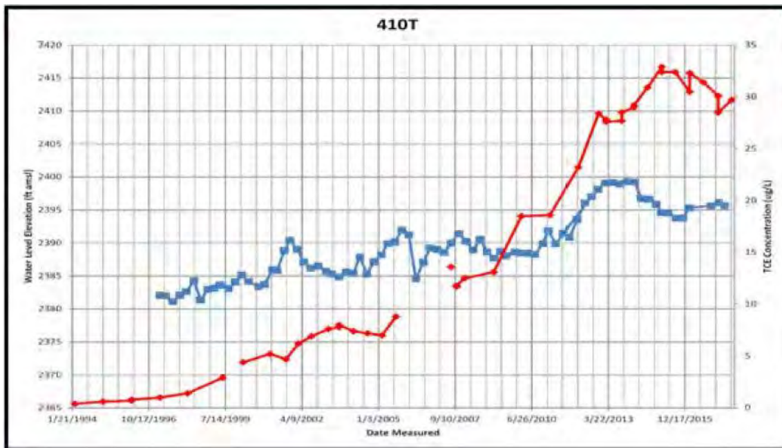
Figure C-8. Well 410T Illustrating the Relationship Between Water Levels and TCE Concentrations.
