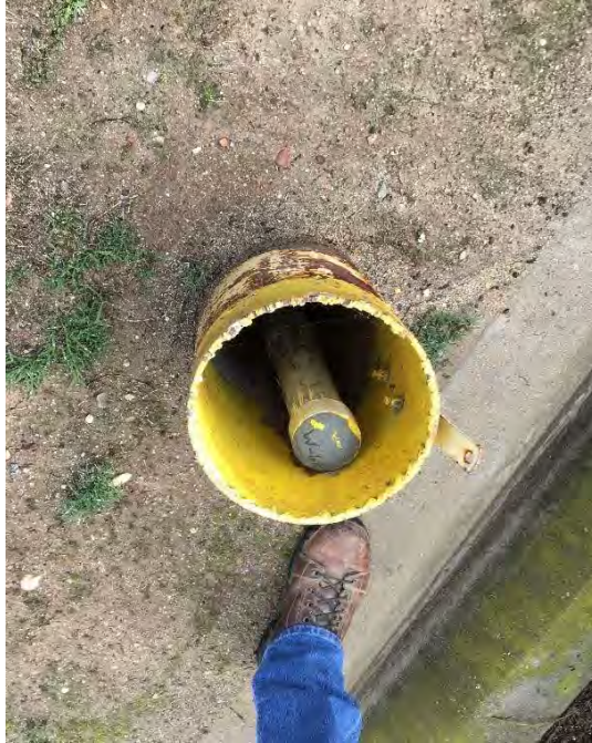
Photograph 6. Well W-6D observed in the Ramparts Sumps Area, typical of the above ground monument installed on the Site.
