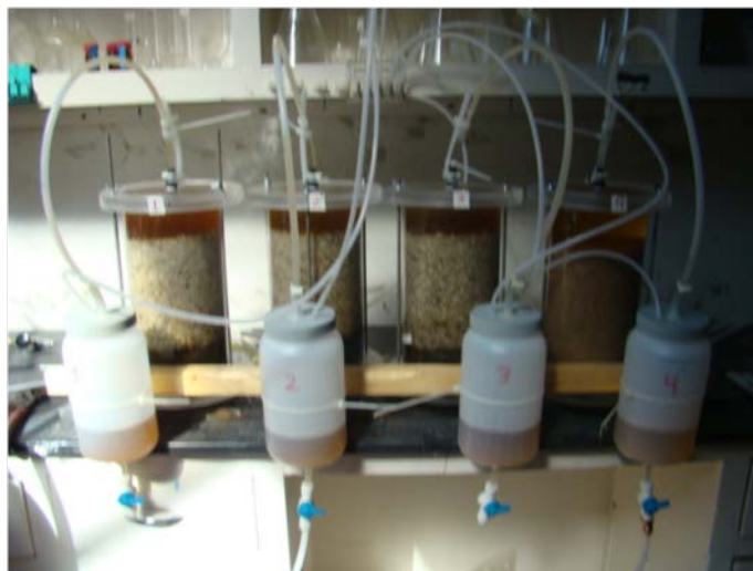
Exhibit 2-7. Completed and operational column test setup.
