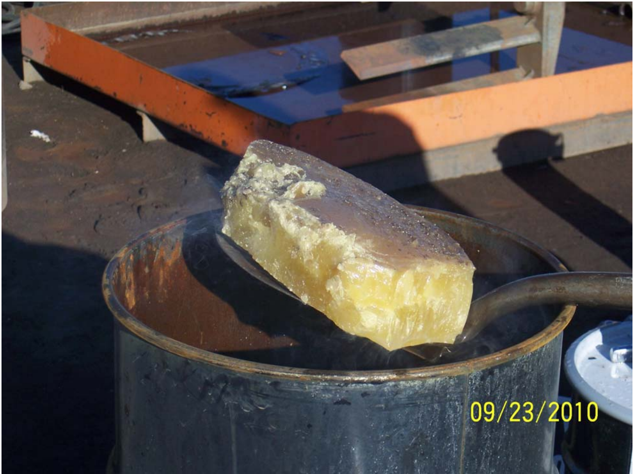
Some of the recovered phosphorus immediately after lifting from the water cap.
