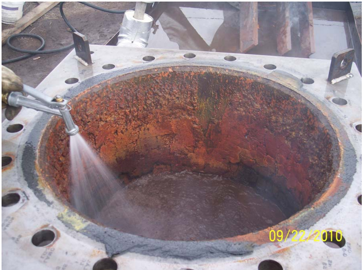
Still residue after Run #3 indicating red phosphorus
