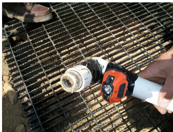
Exhibit 2-8. Camera lens installed in PVC pipe fitting to obtain horizontal recordings
