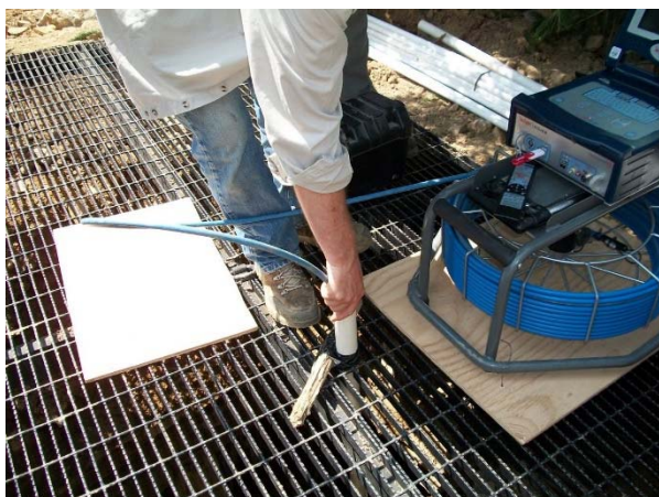
Exhibit 2-7. Inserting PVC guide pipe and camera into shaft
