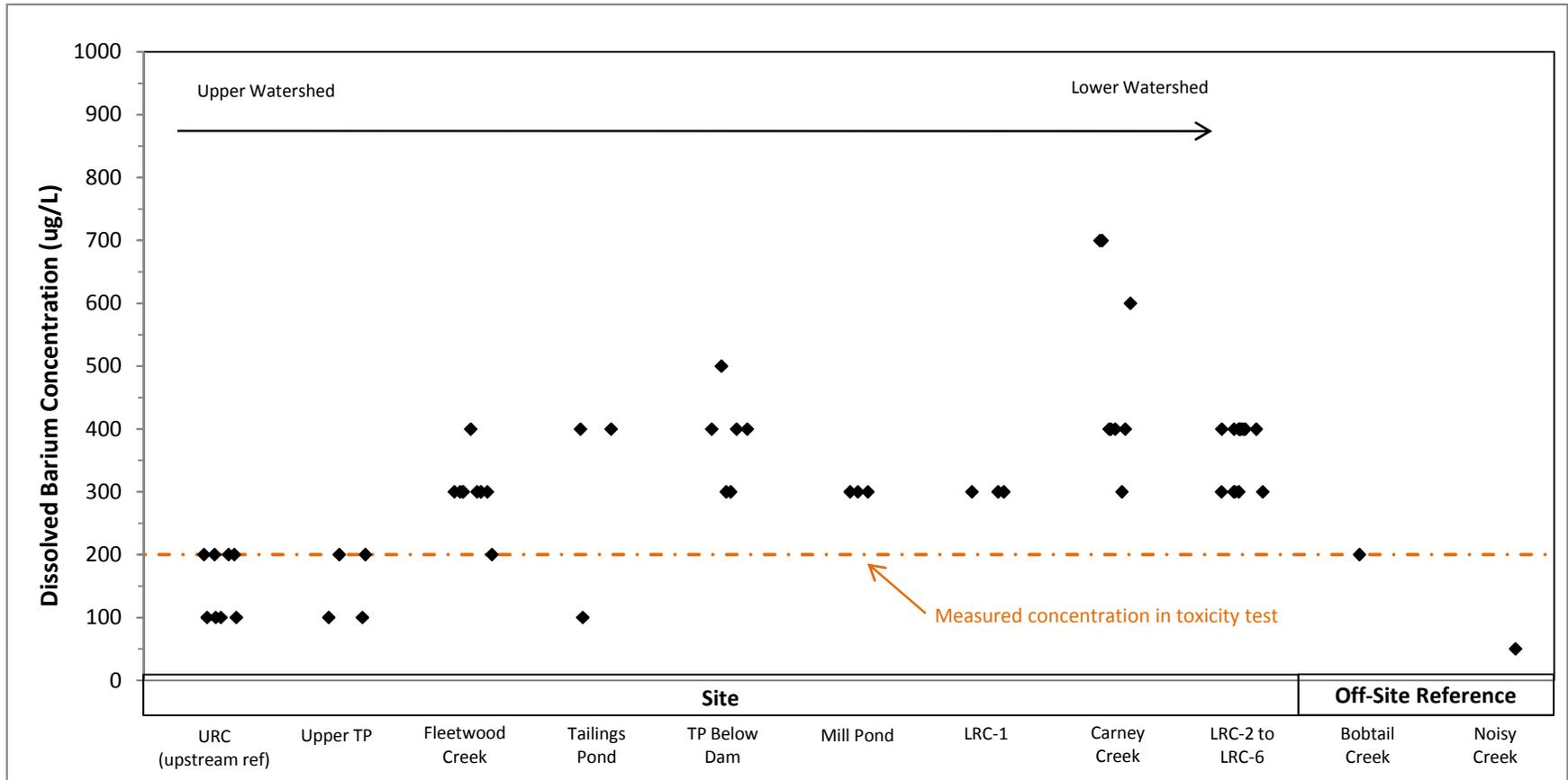
**FIGURE 8-2. COMPARISON OF MEASURED SEDIMENT CONCENTRATIONS IN TOXICITY TEST SAMPLES TO OTHER OU3 SITE LOCATIONS**
