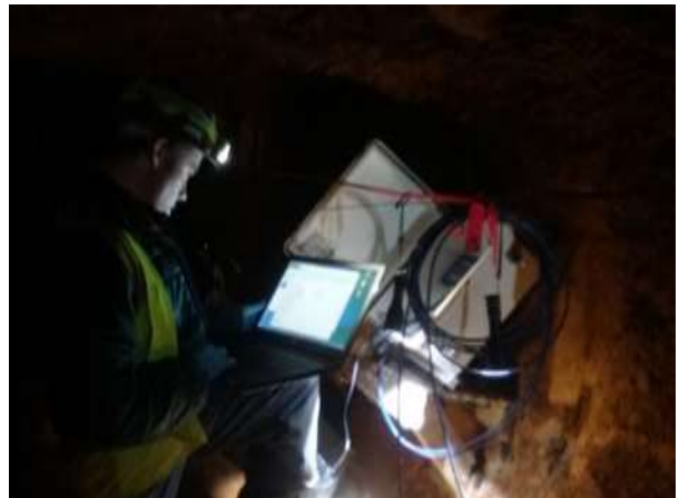
Photos 5-6: R&B mine discharge pipe flow sensor and data logger station.
