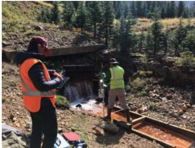
Photo 8: Natalie Occidental mine discharge custom flume
