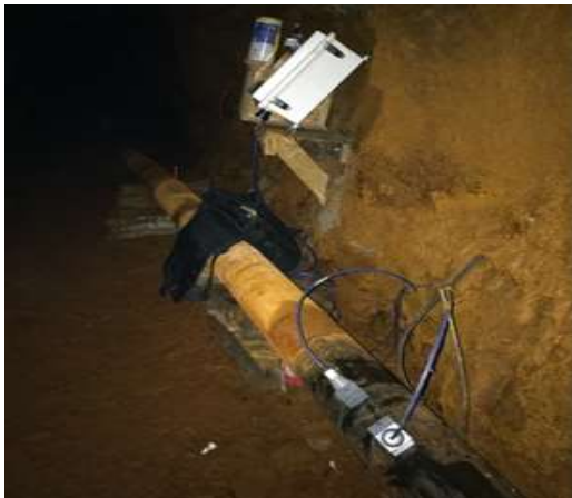
Photos 5-6: R&B mine discharge pipe flow sensor and data logger station.
