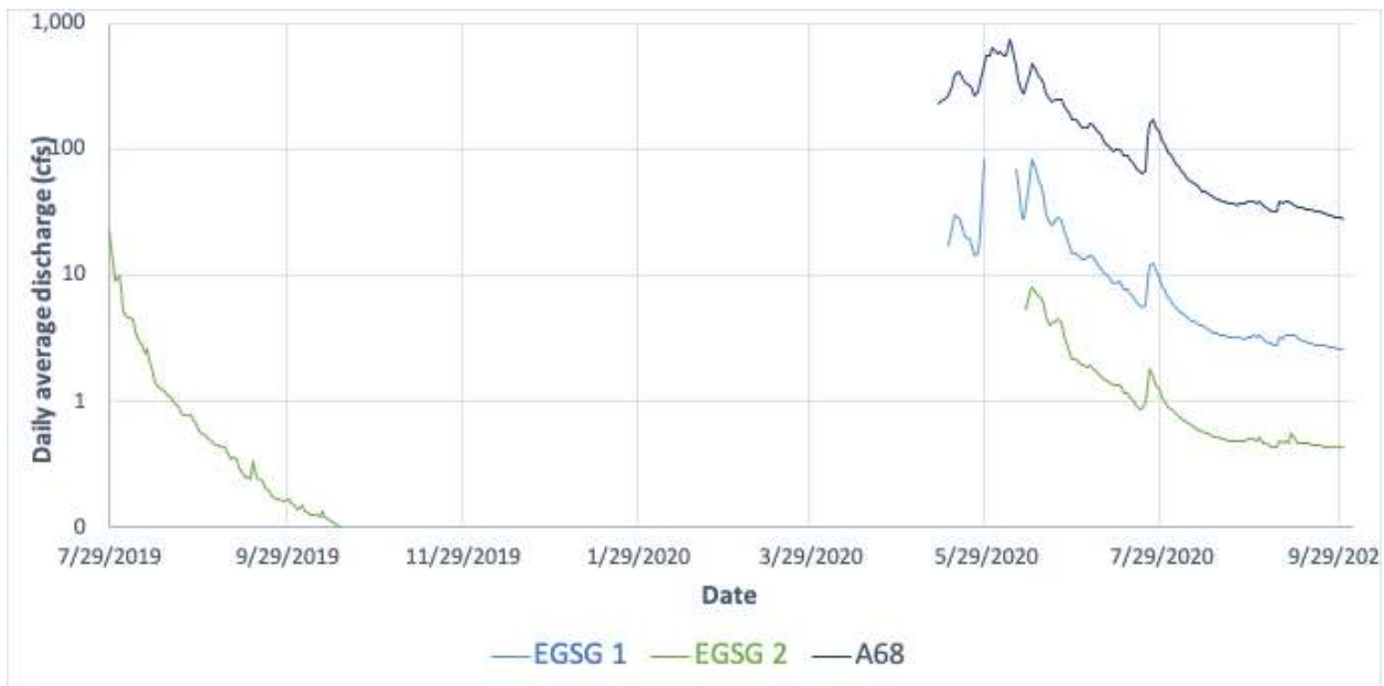
Figure 7: Daily mean discharge for Eureka Gulch stream gages in 2019 and 2020. The USGS gage Animas River above Silverton (A68) is plotted for reference. Discharge plotted on log scale for clarity.
