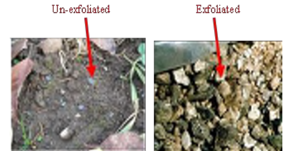
Photo of raw (left) and processed (right) vermiculite. View samples at the EPA Info Center.
