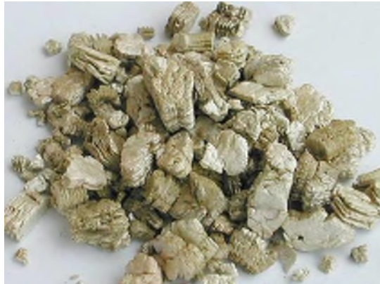
Processed vermiculite often seen as insulation.
