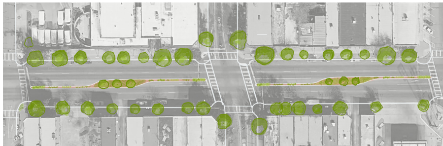
Northern Avenue commercial street with a landscape median and pedestrian bump-outs.
