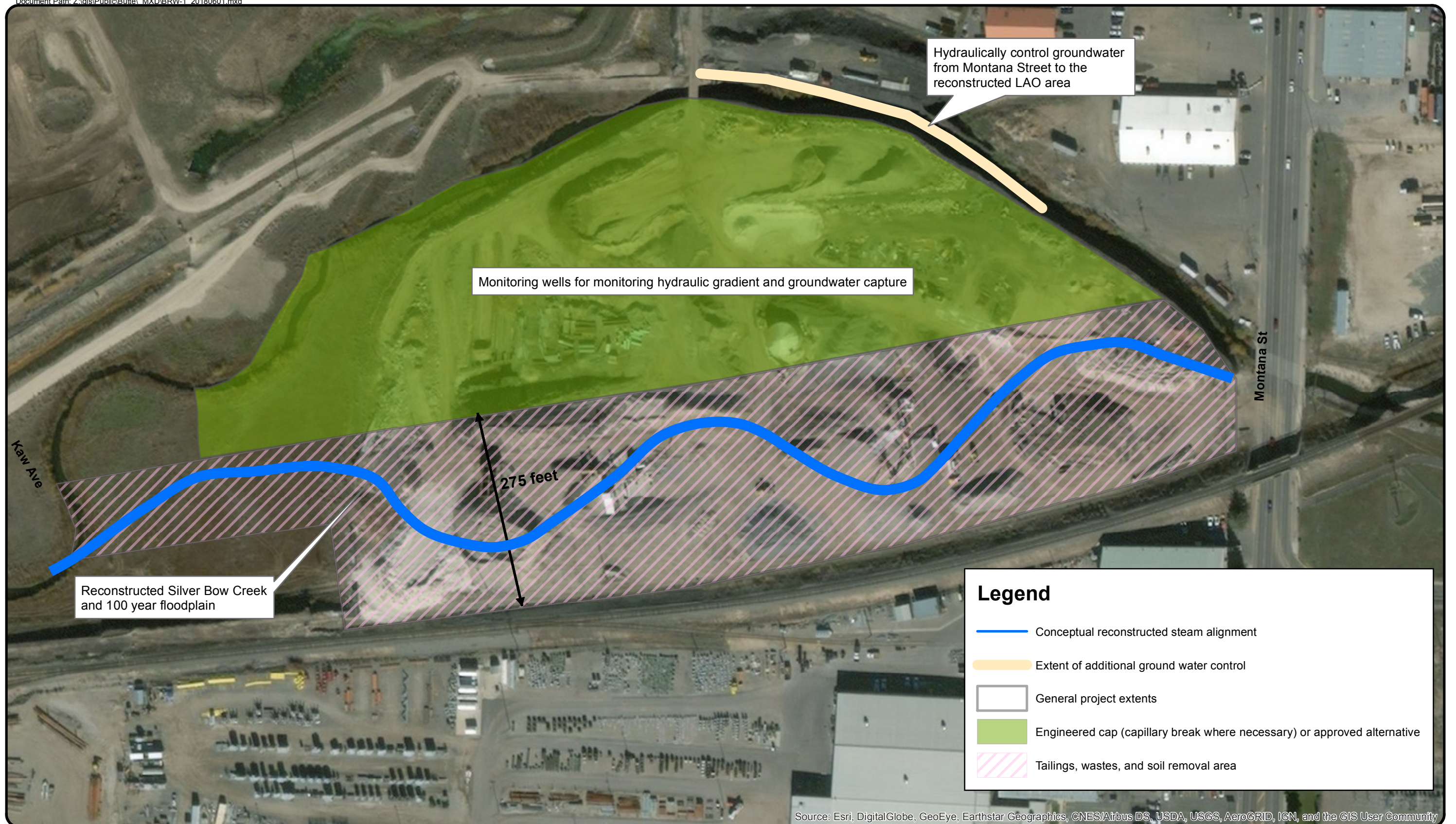
Figure BRW-1 Butte Reduction Works Smelter Area Remedial Action Plan
