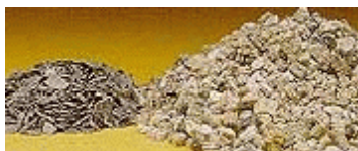
Raw and Popped Vermiculite Ore
