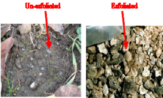
Photo of raw (left) and processed (right) vermiculite. View samples at the EPA Info Center.
