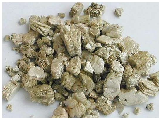
Processed vermiculite often seen as insulation.
