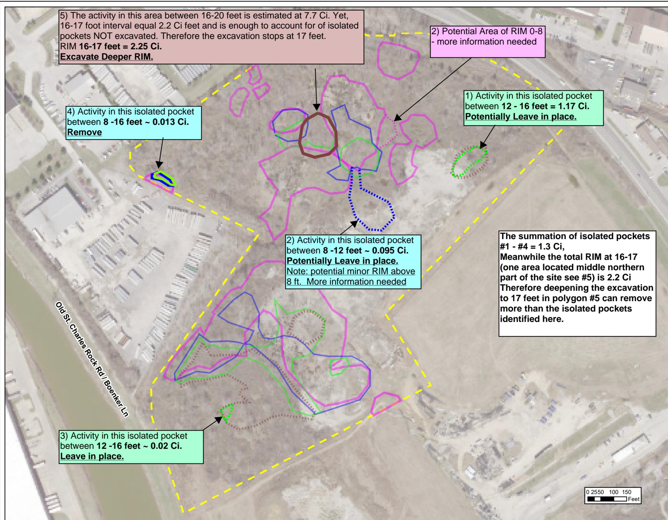
5) The activity in this area between 16-20 feet is estimated at 7.7 Ci. Yet, 16-17 foot interval equal 2.2 Ci feet and is enough to account for of isolated pockets NOT excavated. Therefore the excavation stops at 17 feet.
