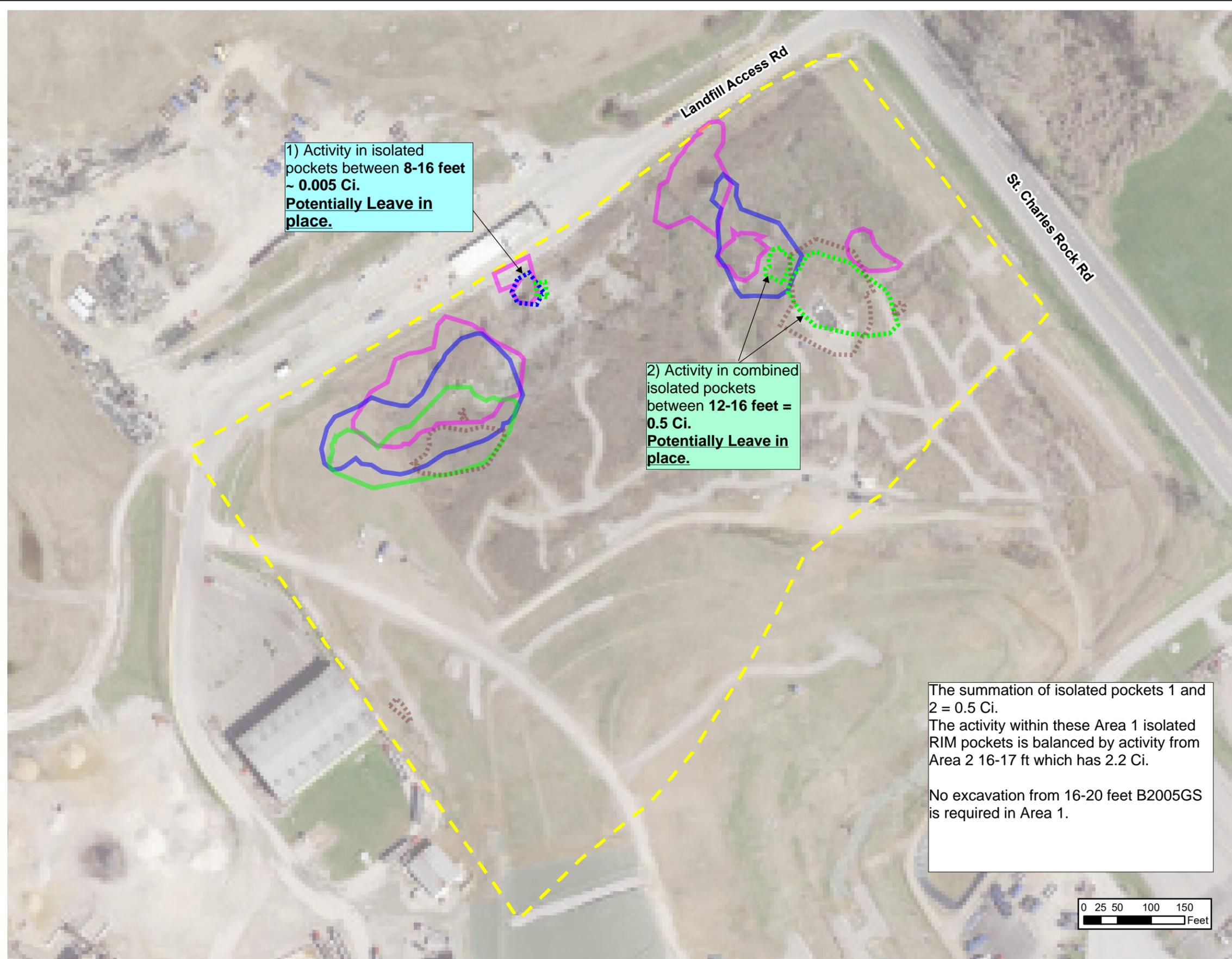
1) Activity in isolated pockets between 8-16 feet ~ 0.005 Ci. **Potentially Leave in place.**
